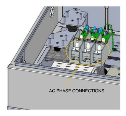
Figure 3-14 AC Connections - Neutral and Ground (Left) and AC Phases (Right)
