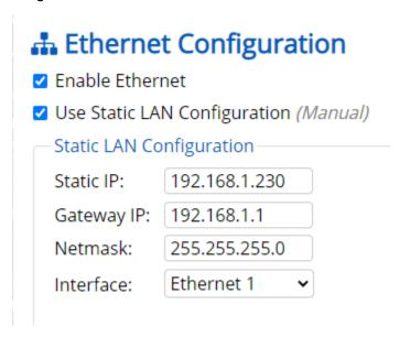
Figure 5-5 Static IP Configuration
