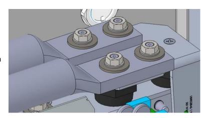
**Figure 3-16 DC Conductor Termination**
