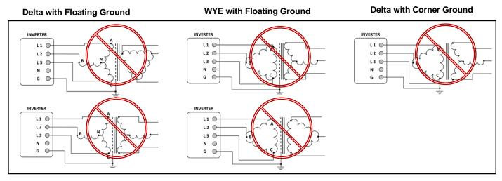
**Figure 3-111 Prohibited Transformer Configurations**
