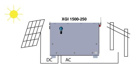
Figure 2-1 Inverter Usage
