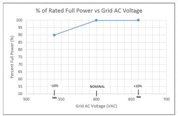
Figure 10-1 Derating with AC Voltage
