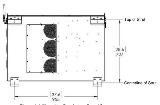
Figure 3-3 Mounting Brackets - Rear View
