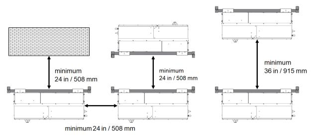
Figure 3-2 Inverter Minimum Spacing and Mounting - Top View
