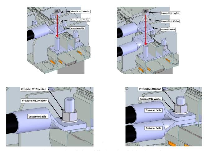
Figure 3-13 Installation of Single or Parallel Conductor Sets
