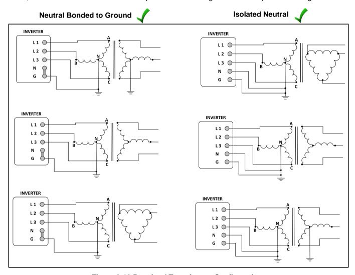
**Figure 3-10 Permitted Transformer Configurations**
