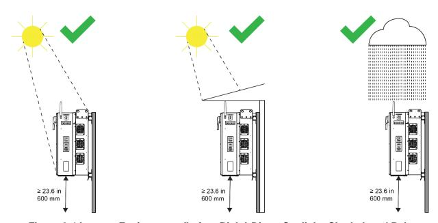
Figure 2-4 Inverter Environment (Left to Right) Direct Sunlight, Shaded, and Rain
