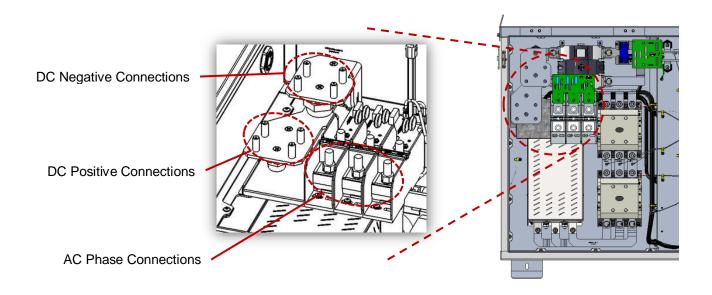
**Figure 3-8 Wiring Box Power Connections**
