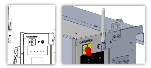
**Figure 3-18 Mounting the Antenna**
