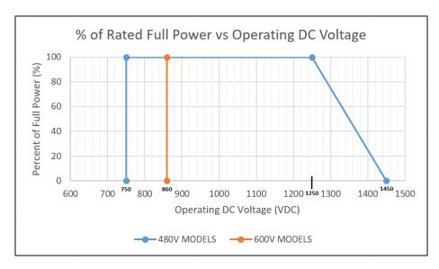
Figure 10-2 Derating with DC Voltage
