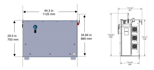
**Figure 3-1 Inverter Dimensions**
