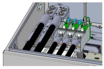
Figure 3-15 DC Connections from a Solectria CR1500 Remote Combiner
