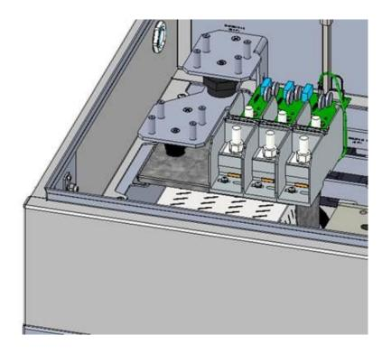
**Figure 9-1 Inverter Wiring Compartment**
