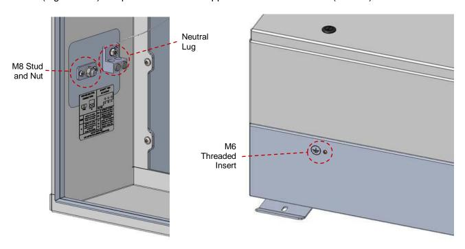
Figure 3-12 Ground Connection Inside and Outside Inverter and Neutral Lug
