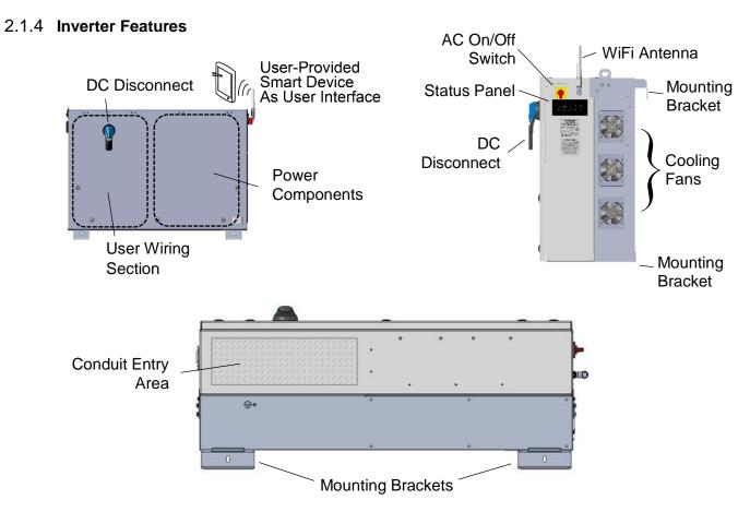
Figure 2-3 SOLECTRIA XGI 1500 Inverter Features: Front (Left), Right Side (Right), and Bottom (Bottom)
