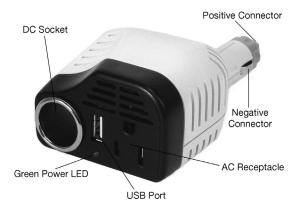
All inverter functions require connecting the Inverter's DC plug into a powered cigarette lighter or 12 volt accessory outlet. The green LED will light up when the inverter is powered. For operations more than 2 hours, make sure the car engine is running.
