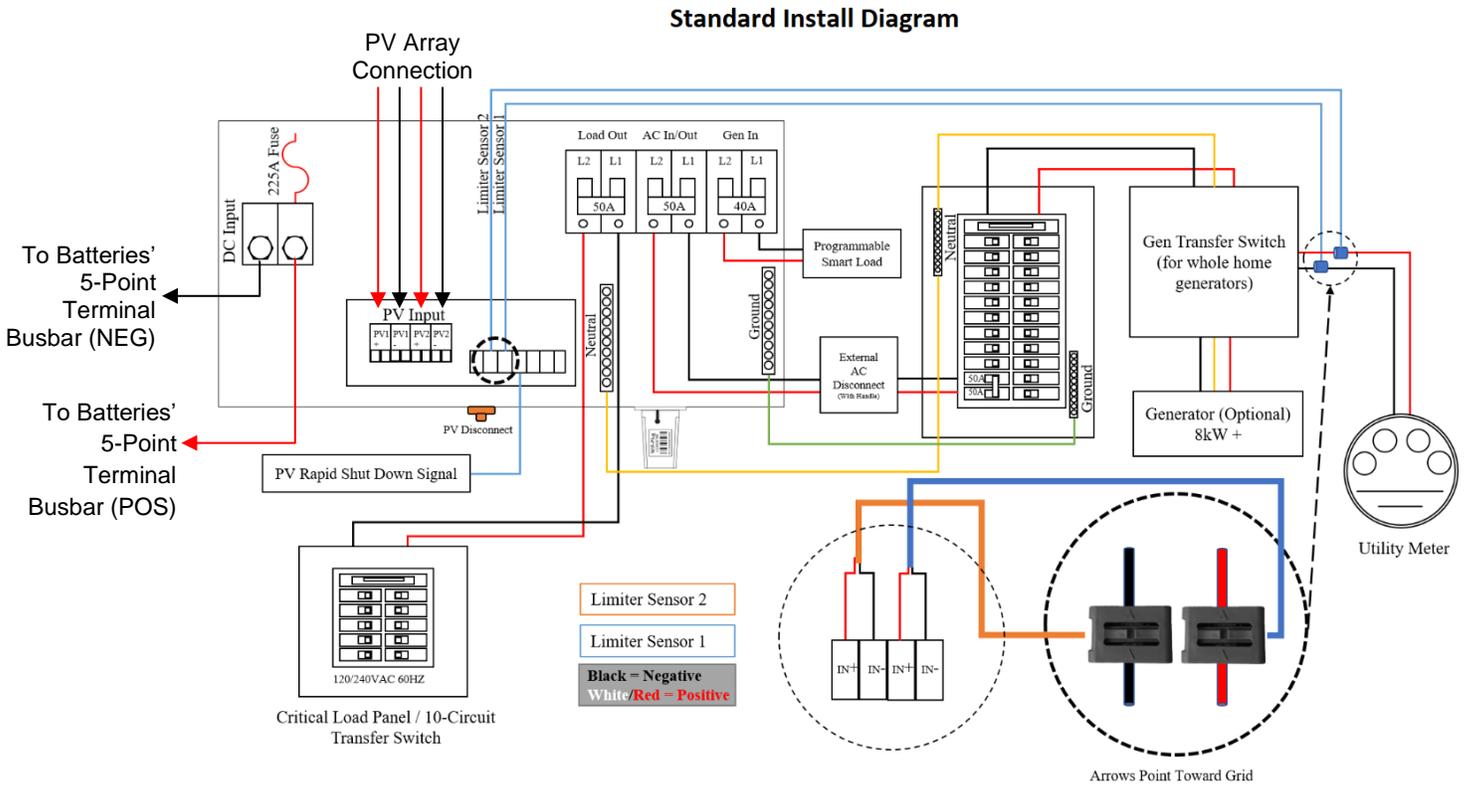
Figure 12.0 – DC Coupled AccESS Sol-Ark Wiring Diagram
