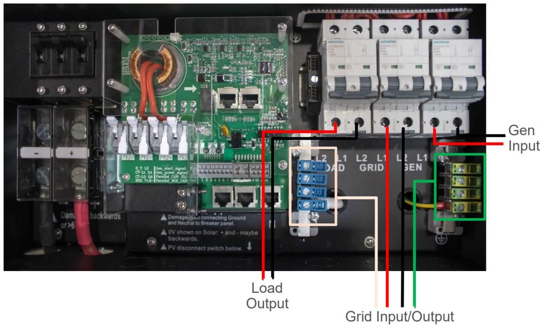
Figure 14.0 - AC Power Input/Output Wiring Connection Points
