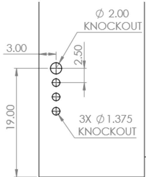
Figure 5.0 – AccESS Cabinet Knockouts (sides)
