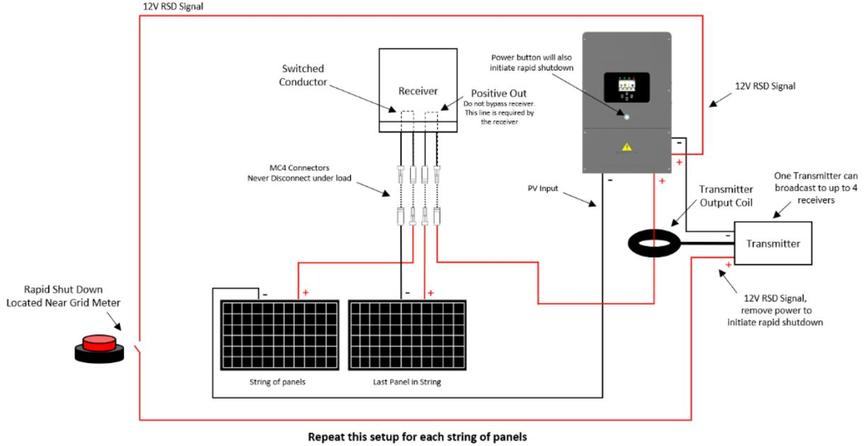
**Note: If parallel systems: the RSD Signals for all systems must be in parallel and pass through the same RSD button**
