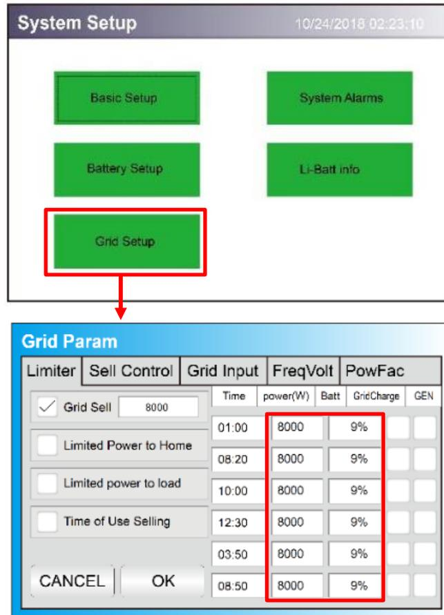
Figure 21.0 – Limiter Tab in Grid Setup Menu
