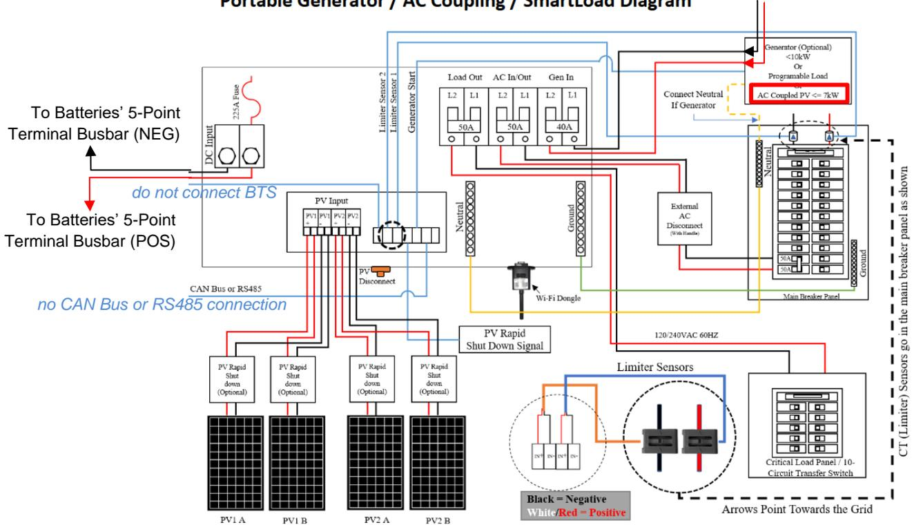
Figure 13.0 – AC Coupled Access Sol-Ark Wiring Diagram
