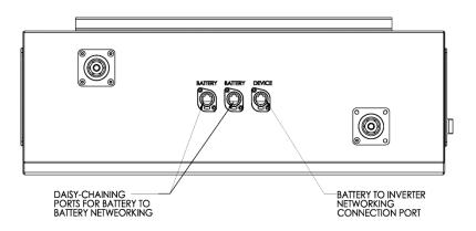
In a string of batteries, the two batteries at the ends of the communication chain will have a cable occupying only one of the "daisy-chaining" ports in the SimpliPHI battery. On each of these two batteries, the communication port not occupied by a cable will need a 1200hm terminator plug installed in the open port (see photo). One terminator plug is included per SimpliPHI battery.
