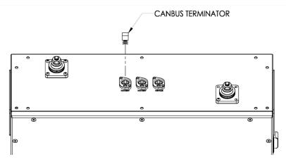
The maximum number of SimpliPHI batteries that can be connected in a single system is 72, with a maximum total connected distance of 40m (131 feet) from the first SimpliPHI battery module to the last SimpliPHI battery module. While one 4' CAT5 networking cable is provided per SimpliPHI battery, shorter networking cable for daisy-chaining the batteries may be used.
