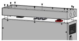
**Step 2:** Complete all wiring connections for battery terminals and communications cables. Use 1" conduit to route 4/0 battery cables and battery communications cables using 1" U.S. trade size knockouts on both sides of the conduit box. **Positive cables and negative cables are to be run in separate conduit.** It is acceptable to run communication cables in either conduit along with battery cable.
