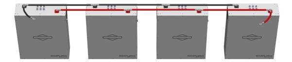
For installations that are larger than 4 batteries, equal sets of batteries not exceeding four batteries per set should be wired to a common busbar or plate. All wire lengths from each SimpliPHI Battery Bank to common busbars or plates should be **identical in length and gauge** in order to balance the load across (all) SimpliPHI Batteries in the installation.
