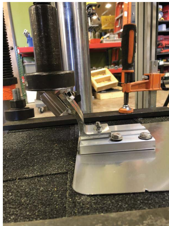
Photo 4: Compressive Load (post-test)
