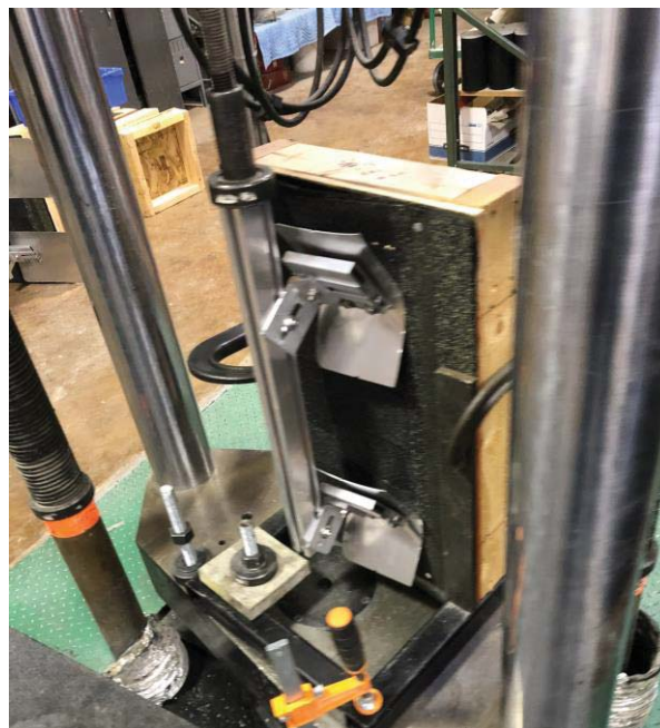
Photo 8: Lateral Perpendicular to Rafter Eccentric Load (post-test)
