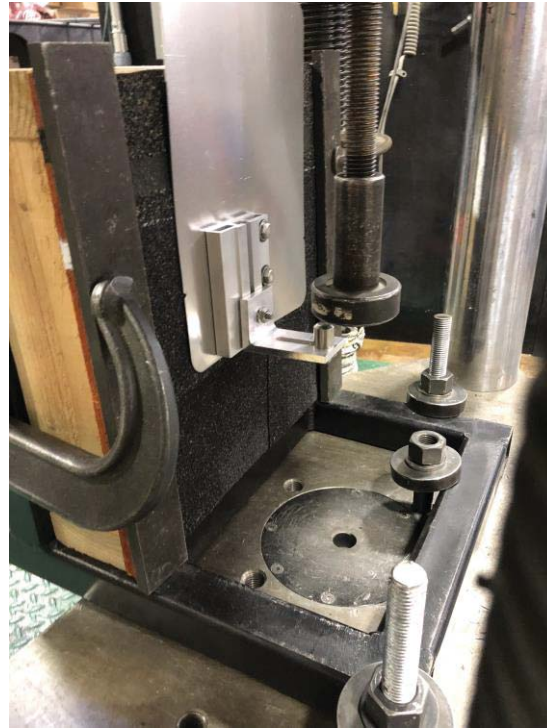
Photo 5: Lateral Parallel to Rafter Eccentric Load (pre-test)
