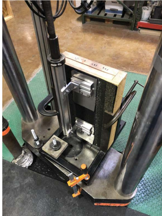
Photo 7: Lateral Perpendicular to Rafter Eccentric Load (pre-test)
