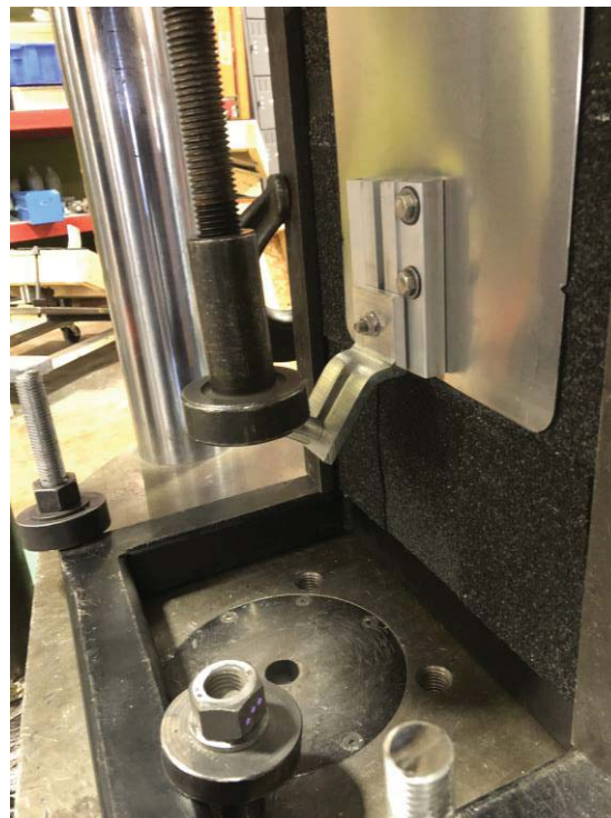
Photo 6: Lateral Parallel to Rafter Eccentric Load (post-test)
