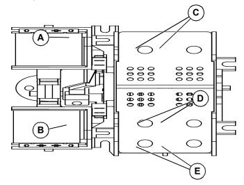
Figure 2-1. Typical Single-Phase ATS Transfer Mechanism
