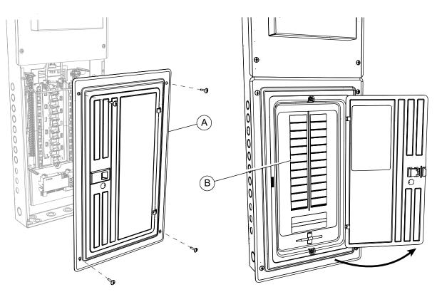
Figure 3-2. Front Panel Assembly and Breaker Knockouts
