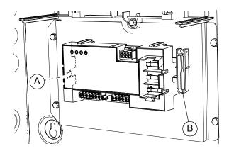
Figure 4-3. SACM Test and Fuse Removal Tool
