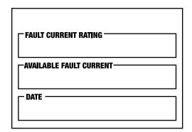
Figure 3-5. Fault Current Label
