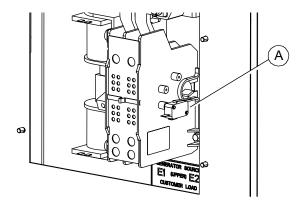
Figure 3-7. Auxiliary Contact
