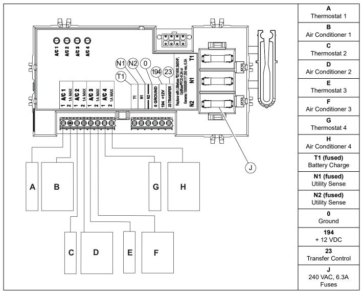
Figure 3-6. Typical SACM Connections
