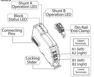
Secure blocks to DIN Rail with cover, clamp or other means provided with host device
