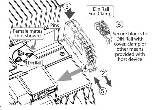
After wiring, tighten the terminal connector screws to 5 in-lb (0.56 N-m) of torque. **Connect the battery to power the host device-relay block system.**
