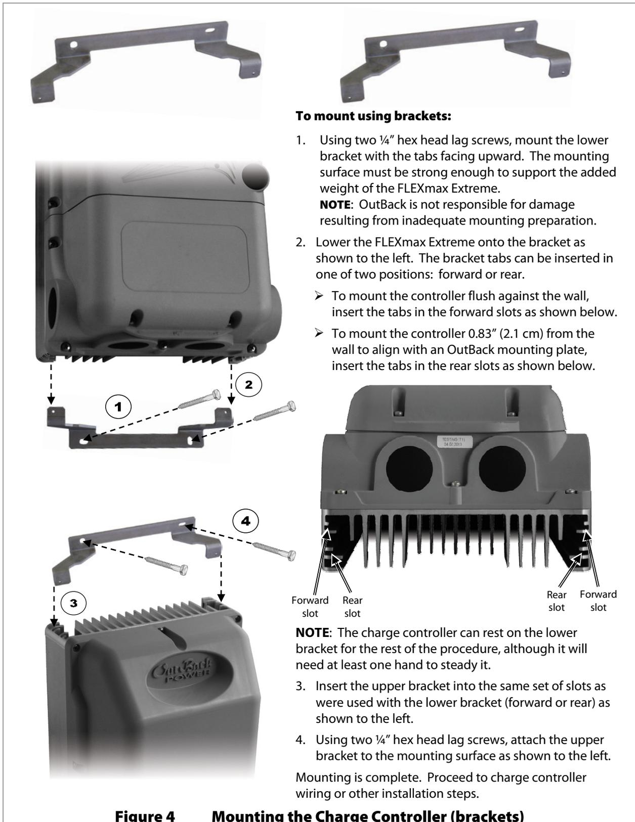
**Figure 4** Mounting the Charge Controller (brackets)
