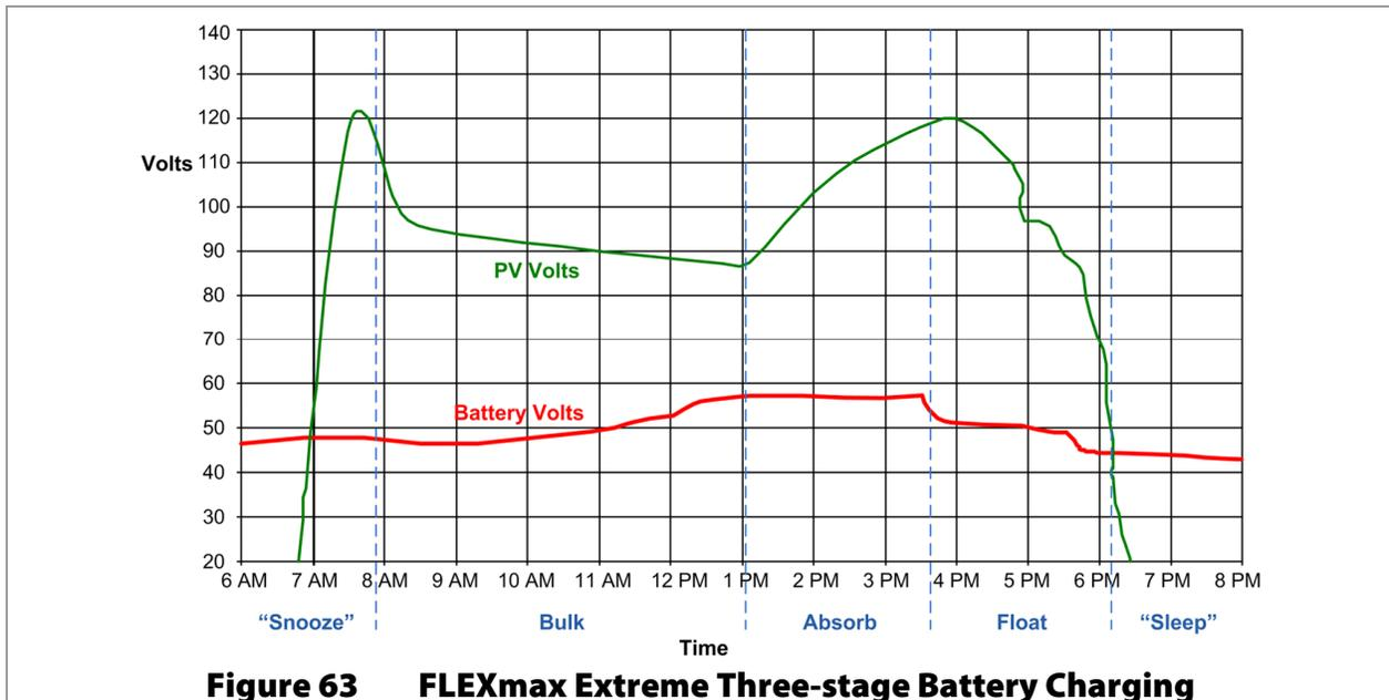
**Figure 63 FLEXmax Extreme Three-stage Battery Charging**
