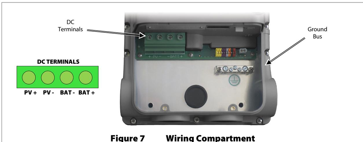
**Figure 7** Wiring Compartment
