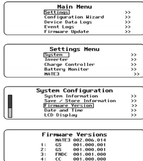
**Figure 47 Reading the Firmware Revision**
