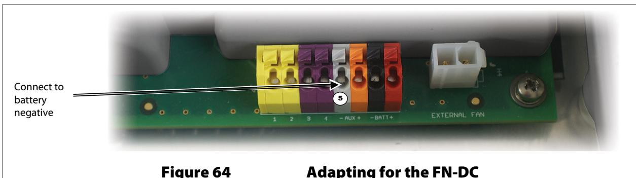
**Figure 64 Adapting for the FN-DC**
