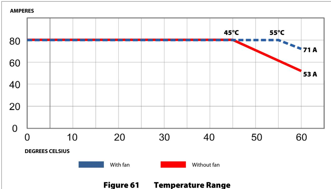
In standard installations, the FLEXmax Extreme can operate at its full 80-amp capacity at ambient temperatures up to 45°C (113°F). Above this temperature, its output is derated as shown in Figure 61. At 60°C (140°F), the output is derated to a maximum of 53 Adc. The controller is not rated for operation above this temperature.
