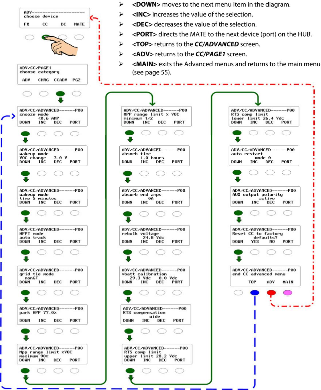
**Figure 58 ADV Menu for the Advanced Charging Features**
