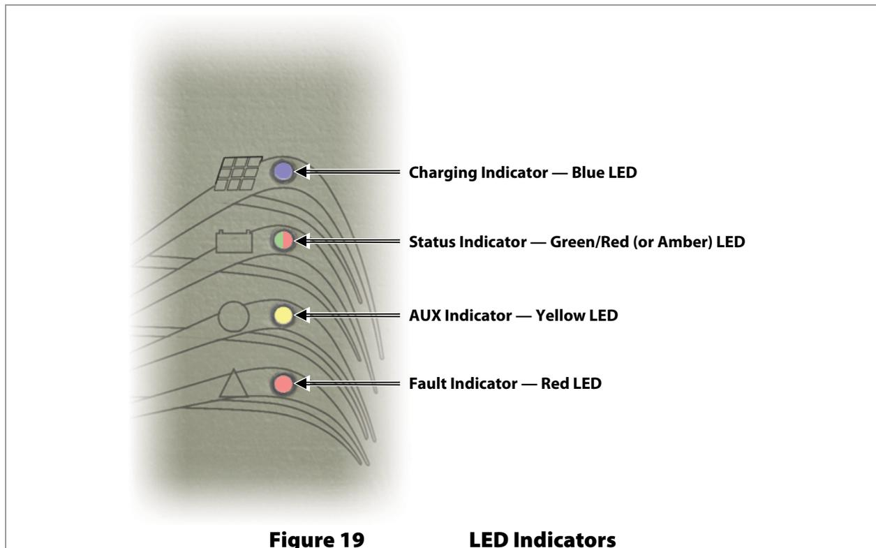
The FLEXmax Extreme charge controller has no graphical display. It is equipped with four LED indicators that show the charge controller's condition.
