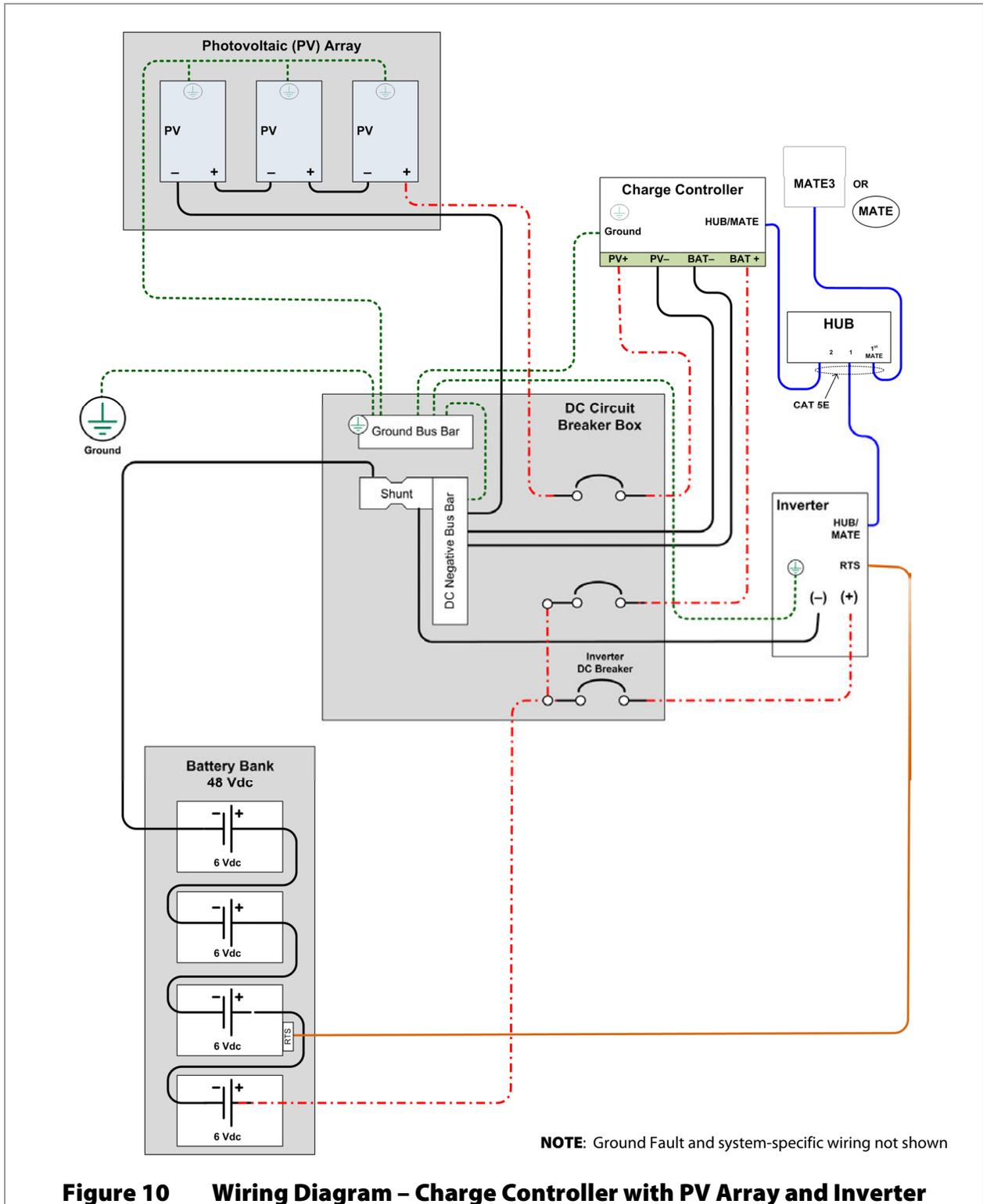
**Figure 10** Wiring Diagram - Charge Controller with PV Array and Inverter
