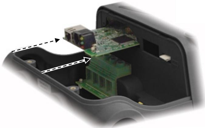
2. Insert the AXS Card onto the rails on each side of the compartment. Slide it in until the card presses firmly onto the connector at the rear of the compartment.
