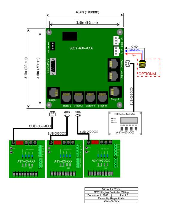
Note: Three stages shown. One additional display and three additional controls can be connected. Relay contacts are for external alarm relay. Computer connection is for certain legacy systems only.
