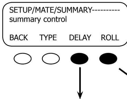
In the SETUP/MATE/SUMMARY screen, press the <DELAY> soft key; this will take you to the *sum screen delay time* screen. Pressing the <ROLL> soft key leads to the *sum screen roll rate* screen.
