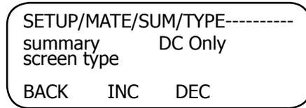
**DC Only**—displays the DC SUMMARY screen. Pressing the <INC> soft key opens the *DC Only Simple* screen.
