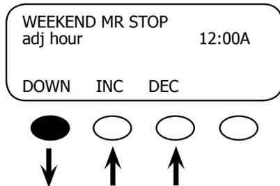
Adjust the hour settings using the <INC> and <DEC> soft keys. Press the <DOWN> soft key when finished to go to adj min screen to change the minutes.
