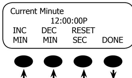
Adjust the minutes by pressing the <INC MIN> or <DEC MIN> soft keys as needed. Pressing the <RESET SEC> soft key begins the seconds count at zero. Pressing the <DONE> soft key returns the MATE to the SETUP/MATE/CLOCK screen.
