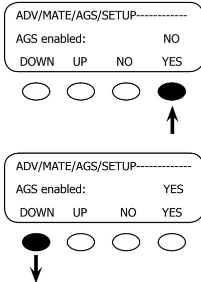
This is the overall control for the AGS Mode. If AGS is not enabled, none of the AGS settings or controls will work. Enable the AGS first by pressing the <YES?> soft key and then establish your settings.
