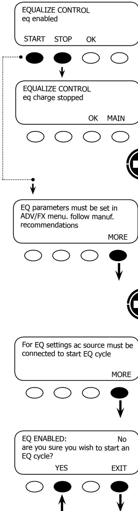
Pressing <EQ> on the CHARGER MODE CONTROL screen brings up the EQUALIZE CONTROL screen
