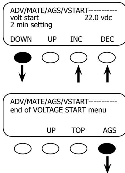
If the battery voltage falls below this set point, a 2-minute timer starts to count down. Upon reaching zero, a start command is sent to the generator even if it is currently Quiet Time. Use the <INC> and <DEC> soft keys to change the default settings. When finished, press the <DOWN> soft key to go to the *end of VOLTAGE START* menu.
