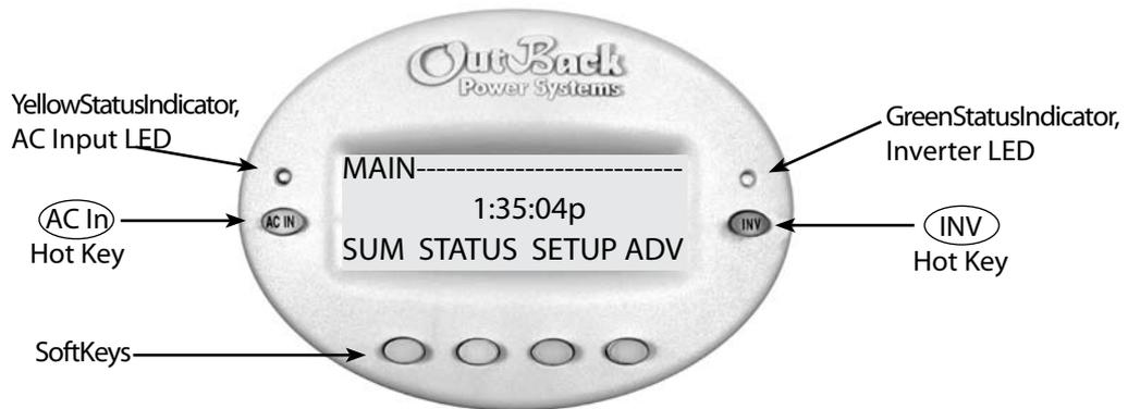
Six buttons or keys navigate the MATE and change its settings:
