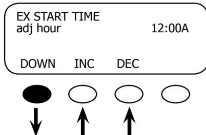
After adjusting the exercise start time hour, press the <DOWN> soft key and go to the *adj min* screen.
