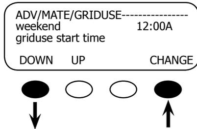
This setting is the time during the weekend (Saturday and Sunday) that a <USE> will be issued to an FX system, allowing the FX to connect to the AC input source. The time displayed is the default setting. To change the time press the <CHANGE> soft key and adjust the time as you would for a weekday setting. Press the <DOWN> soft key to view the *weekend griduse stop* screen.
