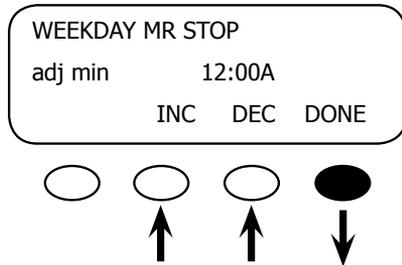
Adjust the minutes using the **<INC>** and **<DEC>** soft keys. When finished, press the **<DONE>** soft key to return to the ADV/MATE/AGS/MR *weekday must run stop time* screen.
