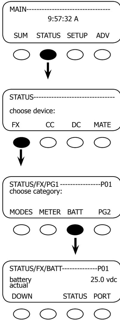
The top line of the MATE display will show the 'path' to the current menu; in this example it is STATUS/FX/BATT-----P01 with "P01" referring to the first port of the HUB.
