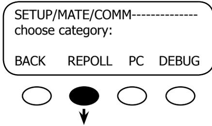
Press the <REPOLL> soft key after a device is added to, moved, or removed from the HUB.
