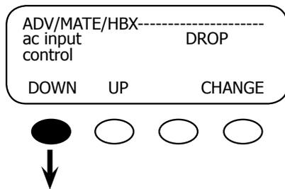
Press the <UP> soft key to return to the *hbx-drop grid delay* screen. Press the <DOWN> soft key to open the *end of HBX menu* screen.
