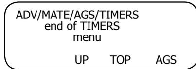
This is the final TIMERS screen. Press the <AGS> soft key to view the final AGS screen.
