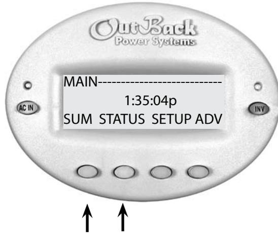
Press the first two soft keys from any screen to return to the MAIN screen.
