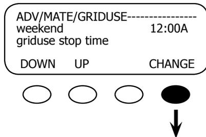
This setting is the time during the weekend (Saturday and Sunday) that a **DROP** will be issued to the FX system, forcing the FXs to disconnect from the AC input source. The time displayed is the default setting. To change the time press the <CHANGE> soft key and adjust the time as you would for a weekday setting.
