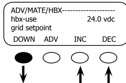
This is the voltage set point that allows the FX to connect to (USE) AC power. The battery voltage must remain below the voltage listed on the screen—24.0 vdc in this case—for the amount of time programmed by the HBX-USE GRID DELAY (see next screen) before a USE command is issued. Use the <INC> and <DEC> soft keys to change the voltage set point. Press the <DOWN> soft key to proceed to the next screen.
