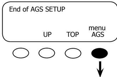
In the End of the AGS SETUP screen Press the <menu AGS> soft key for more AGS programming.
