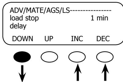
This setting is the delay time the total system AC load must remain below the Load Stop kw before the generator is stopped. It is adjustable from 1 to 240 minutes using the <INC> and <DEC> keys. Pressing the <DOWN> soft key leads to the *end of the VOLTAGE START* menu screen.
