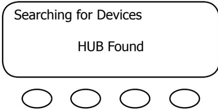
The MATE has found the HUB and will automatically go to the Port Assignment screen.
