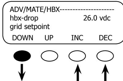
This set point shows the voltage—26.0 VDC is the default for a 24V system—at which the FX will DROP its AC input source. The battery voltage must remain above this voltage for the amount of time set by HBX-DROP GRID DELAY (next screen) for a DROP to be issued. Press the <DOWN> soft key to proceed.
