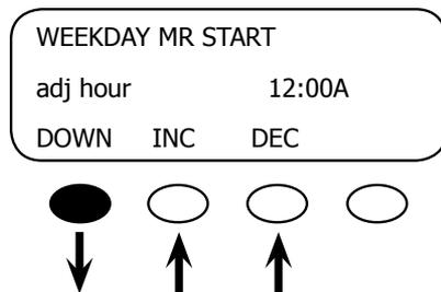
Adjust the weekday must run start time minutes with the **<INC>** and **<DEC>** soft keys. Press the **<DOWN>** soft key to view the *adj min* screen.
