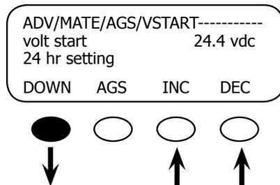
If the battery voltage falls below this set point, a 24 hour timer starts counting down. Upon reaching zero, a start command is sent to the generator unless it is currently Quiet Time. To change the default settings, use the **<INC>** and **<DEC>** soft keys. When finished, press the **<DOWN>** soft key to go to the *volt start 2 hr setting* screen.
