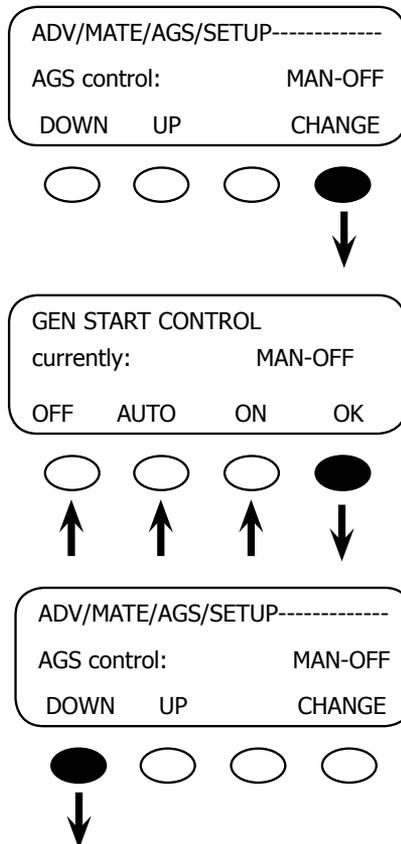
This screen allows the AGS Mode to be changed. Pressing <CHANGE> brings up a screen that allows the user to switch choose from three AGS control modes sown below.
