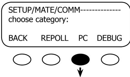
The next communication function deals with the MATE/personal computer interface. Press the <PC> soft key to enable or disable the MATE's RS232 communications port.
