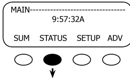
Press <STATUS> on the Main menu to access the STATUS menu. STATUS contains all the meters and mode displays for OutBack products connected to the MATE.
