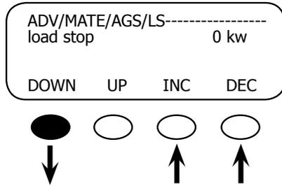
An AGS stop command will be issued when the total AC load of all the FXs connected to the MATE falls below this setting for the amount of time set with *load stop delay* (next screen) as long as the generator was started due to Load Start. This setting excludes any FX charger current for its AC load calculation. The setting can be changed using the <INC> and <DEC> soft keys. Pressing the <DOWN> soft key leads to the *load stop delay* screen.
