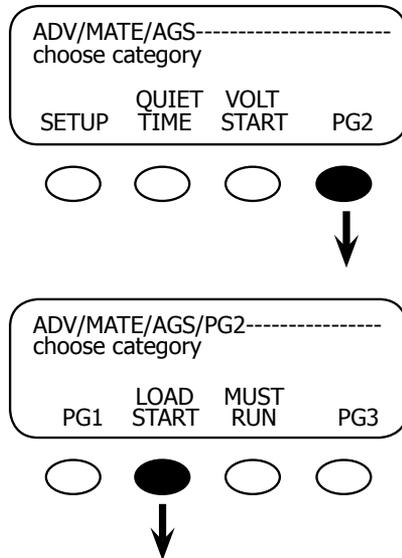
Go to the ADV/MATE/AGS screen and press the <P2> soft key.
