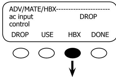
Enable HBX by pressing the <HBX> soft key. The screen now indicates the MATE is running in HBX mode by displaying the current state, USE or DROP followed by HBX.
