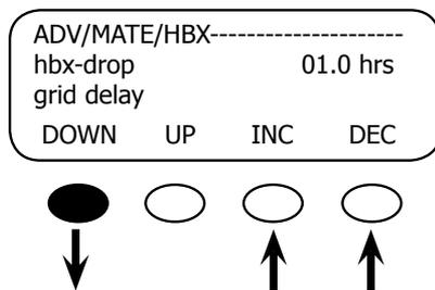
This set point is the amount of time—01.0 hrs in this case—battery voltage must remain above the HBX-DROP GRID SET POINT (see previous screen) before a DROP command is sent. It can range from 00.1 hrs to 24.0 hrs in 0.1 hour increments. These increments are adjusted using the <INC> and <DEC> soft keys. Press the <DOWN> soft key to proceed.
