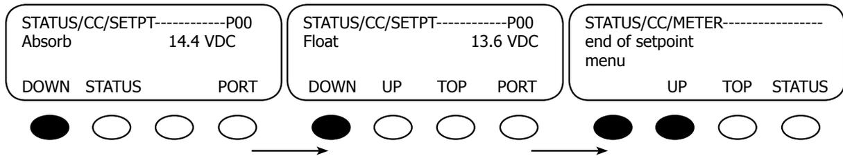
Press the first two soft keys simultaneously to return to the MAIN Menu or press <STATUS> and then press <MAIN> on the STATUS screen.
