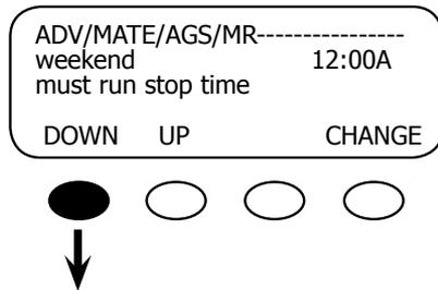
To proceed to the end of MUST RUN menu, press the <DOWN> soft key.
