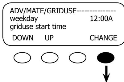
This setting is the time during the week (Monday–Friday) that a USE will be issued to the FX system, allowing it to connect to the AC input source. The time displayed is the default setting. To change the time on the *adj hour* screen, press the <CHANGE> soft key
