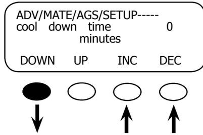
After the FX charging has been disabled, the *cool down time* screen allows the user to adjust the number of minutes the generator will cool down before being shut off. This time should follow the manufacturer's recommendations. Press the <DOWN> key to view the warm up time screen
