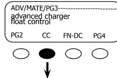
Pressing the <CC> soft key enables charge controller *float state coordination*. This means when a charge controller finishes a bulk charge and moves into float charge, the MATE directs any other charge controllers into a float charge as well. Pressing the <NO> soft key disables *float state coordination*.
