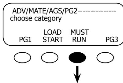
From the ADV/MATE/AGS/PG2 screen, press the **<MUST RUN>** soft key and open the ADV/MATE/AGS/MR *weekday must run start time* screen.
