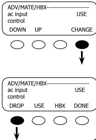
With this screen, HBX Mode can be enabled or disabled. Pressing <CHANGE> allows you to change the current mode in the next screen.
