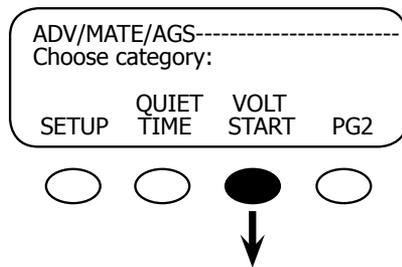
To get to the Voltage Start screen, press the **<VOLT START>** soft key on the ADV/MATE/AGS screen.
