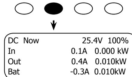
The FLEXnet DC summary screens display the battery state of charge, including the day's minimum, the current DC voltage, and the in and out kilowatt hours and amp hours. All the FLEXnet DC summary screens are explained in the *FLEXnet DC User's Guide* which comes with that component.
