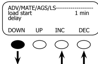
This setting is the delay time that the total system AC load must remain above the load start kw setting (see previous screen), before the generator is started. It is adjustable from 1 to 240 minutes using the <INC> and <DEC> soft keys. After making any adjustments to the delay time, press the <DOWN> soft key to go to the *load stop kw* screen.
