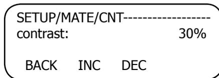
**<INC>** increases the contrast level and **<DEC>** decreases the contrast level. After adjusting the contrast, press the **<BACK>** soft key to return to the previous **SETUP/MATE/PAGE 1** screen.
