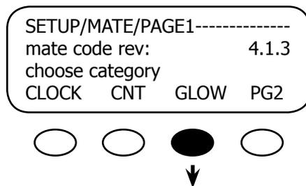
On the SETUP/MATE/GLOW screen, pressing the **<GLOW>** soft key brings up three backlight settings:
