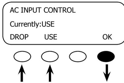
Push the <AC IN> hot key to view the AC status and change to USE or DROP as needed. Pressing the <OK> soft key means you accept the conditions or mode shown on the screen.
