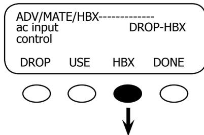
To disable HBX Mode, press the <HBX> soft key again. After disabling HBX, the system remains in whichever state—DROP or USE—it was in while HBX Mode was active. Be sure to reset the DROP or USE to the desired state once it's out of HBX Mode.
