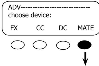
In the ADV menu, push the <MATE> soft key to view the Advanced MATE functions.
