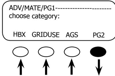
Pressing the <HBX>, <GRIDUSE>, or <AGS> soft keys open their specific advanced functions. Pressing the <PG2> soft key opens the next MATE advanced screen.
