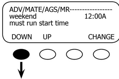
Press the <DOWN> soft key to go to the ADV/MATE/AGS/MR weekend must run stop screen.
