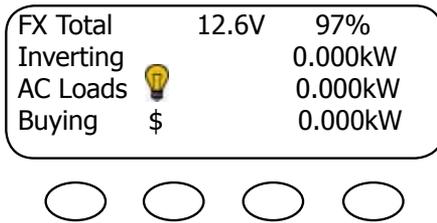
If the MATE has one or more FXs connected to it and does not have a FLEXnet DC as part of the system, an FX Summary screen will be displayed as the Summary default screen. Otherwise, it will follow the FLEXnet DC summary screens.
