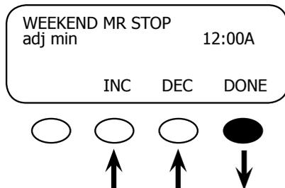
Adjust the minutes settings using the <INC> and <DEC> soft keys. When finished, press the <DONE> soft key to return to the ADV/MATE/AGS/MR weekend: must run stop time screen.
