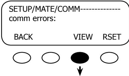
On the DEBUG screen, first press the <VIEW> soft key to bring up a list of HUB ports with a count of communications errors for each port; <RESET> allows you to reset the error counting display (see next screen).
