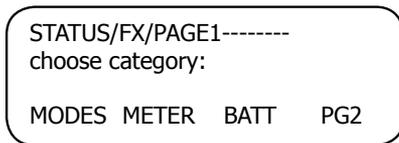
Pressing the <METER> soft key brings up the first METER screen.
