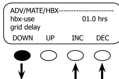
This set point—01.0 hrs in this example—is the amount of time the battery voltage must remain below the HBX-USE GRID SET POINT (above) before a USE command is sent. It can range from 00.1 hrs to 24.0 hrs in 0.1 hour increments. Times are adjusted using the <INC> and <DEC> soft keys. Press the <DOWN> soft key to proceed to the next screen.
