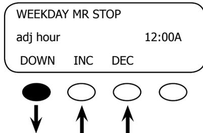
Adjust the hours using the **<INC>** and **<DEC>** soft keys. When finished, press the **<DOWN>** soft key to adjust the minutes.
