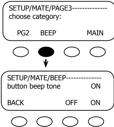
The <**BEEP**> soft key leads to a screen controlling the MATE's beep tone, which is made whenever a key is pressed.
