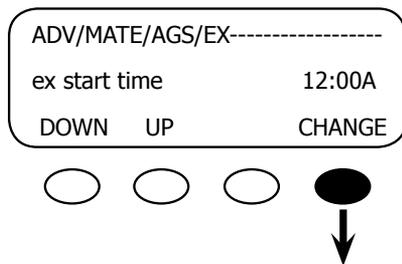
This setting controls the daily exercise start time. Press the <CHANGE> soft key to adjust the hour and minute settings using the <INC> and <DEC> soft keys on the hour and minute screens.
