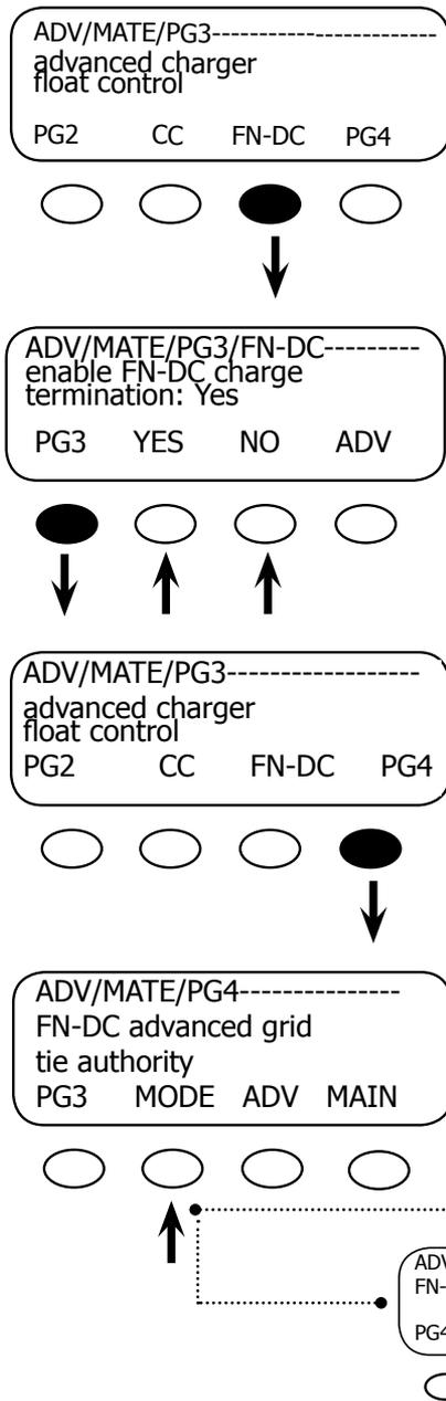
Pressing the <FN-DC> soft key brings up the FLEXnet DC *charge termination* screen.
