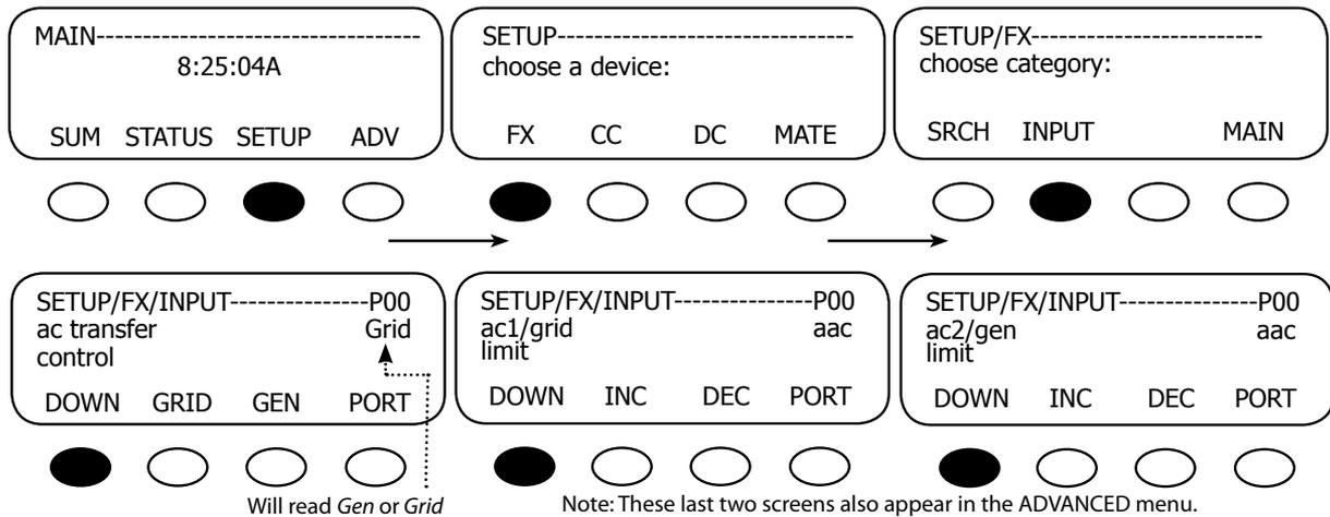
Grid-Use Mode allows programming the times the FX system connects to an AC input source and enables the **USE** mode. The time and date must be accurately programmed for Grid-Use mode to function properly.
