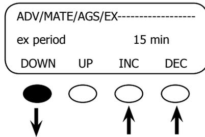
The exercise period screen allows you to set the length of the exercise period using the <INC> and <DEC> soft keys. The MATE offers a range of 1-240 minutes for this period, but check your generator manufacturer's recommendations before setting this period. Press the <DOWN> soft key to exit this screen and go to the ADV/MATE/AGS/EX *end of exercise menu* screen.
