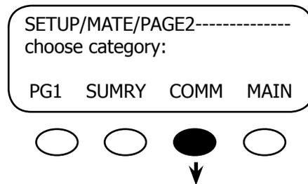
From the SETUP/MATE/PAGE2 screen, press the <COMM> soft key.
