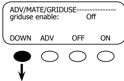
The first GRID-USE screen to appear is the *griduse enable* screen. This screen turns GRID-USE mode ON or OFF.
