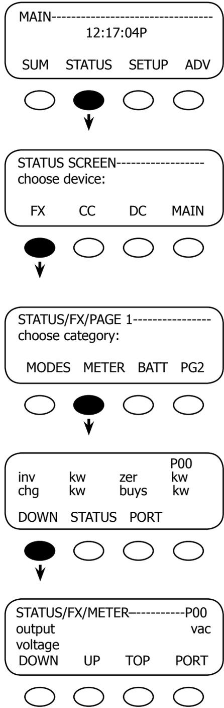
All the screens showing the FX's AC meters are grouped together in one menu branch allowing the user to find the required meter with a minimum of key presses.
