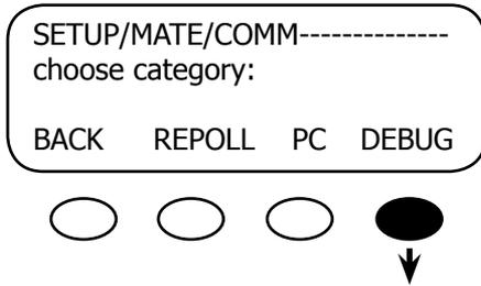
To debug the system, press the <DEBUG> soft key.
