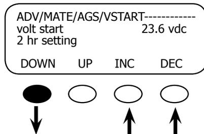
If the battery voltage falls below this set point, a 2 hour timer starts to count down. After reaching zero, a start command is sent to the generator unless it is currently Quiet Time. To change the default settings, use the **<INC>** and **<DEC>** soft keys. When finished, press the **<DOWN>** soft key to go to the *volt start 2 min setting* screen.
