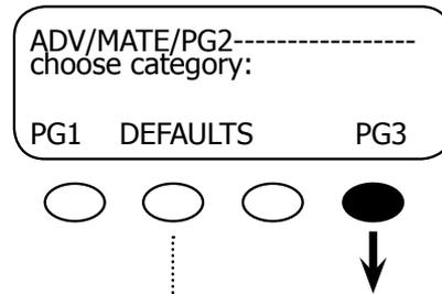
Pressing the <DEFAULTS> soft key brings up the ADV/MATE/DEFAULT screen which allows the user to re-establish all the MATE's factory default values (see pages 96-98). Press the <PG3> soft key to view the next MATE advanced screen.
