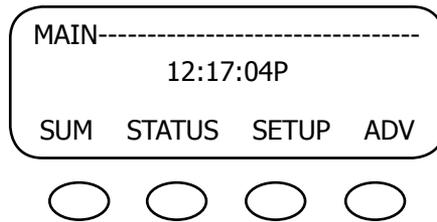
The MAIN screen appears after the MATE detects the HUB (and any devices connected to it) or detects a single device if a HUB is not in use. The MAIN screen is always the same with the exception of the time display. At the bottom of the MAIN screen are the four soft key commands.
