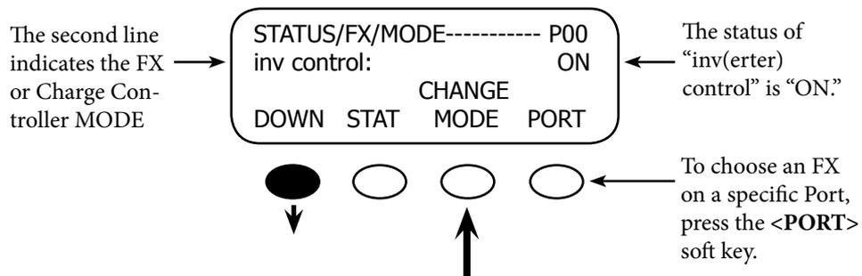
Pressing the <CHANGE MODE> soft key changes the operation of the mode shown on the screen; it does not change to another mode altogether. To change modes, press the <DOWN> soft key.
