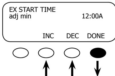
Adjust the minutes and then press the <DONE> soft key to return to the ADV/MATE/AGS/EX *ex start time* screen
