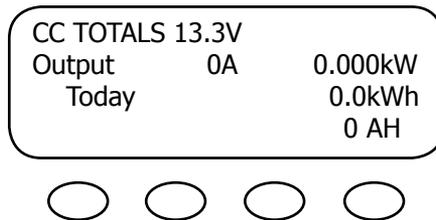
The CC summary applies to all OutBack Charge Controllers. Its screen shows the voltage level of the battery (also non-temperature-compensated) and the amount of power being supplied to the battery. This screen is the default Summary screen if the Charge Controller is directly connected to the HUB. The AH value applies only to the FLEXmax 80 and FLEXmax 60 Charge Controllers.
