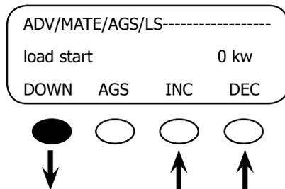
In the *load start kw* screen, an AGS start command will be issued when the total AC load of all the FXs connected to the MATE exceeds this setting for the load start delay (next screen) time. A zero value disables any load start function. <INC> and <DEC> adjusts this setting between 1 - 50kW. After the value has been set, press the <DOWN> soft key to get to the *load start delay* screen.
