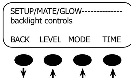
**<LEVEL>** controls the backlight brightness and is adjustable from 0% to 100% using **<INC>** and **<DEC>** soft keys.
