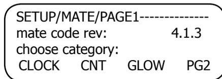
Press the **<CNT>** (**CONTRAST**) soft key from the **SETUP/MATE/PAGE** Setup choices screen. **<CNT>** sets the desired contrast level.
