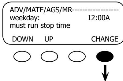
To adjust the start time hour and minute settings, press the **<CHANGE>** soft key.
