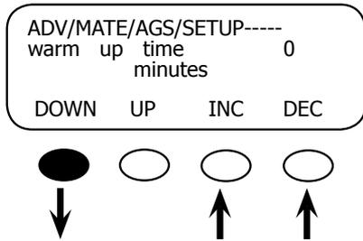
The *warm up time* screen allow the user to adjust the number of minutes the generator will warm up before the FX charging begins. This time should follow the manufacturer's recommendations. Press the <DOWN> key to view the *End of AGS SETUP* time screen
