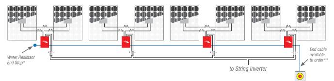
If the array has an odd number of panels, a single panel can be connected directly to the positive (+) and negative (-) panel cables of the FireRaptor.
