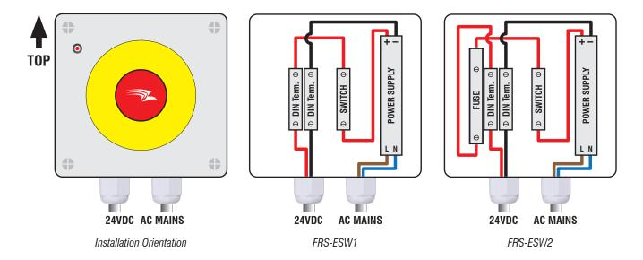
Using appropriate fixings attach the FRS-ESW1 unit vertically to the chosen surface.
