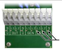
Metal pads are located at these locations. In troubleshooting, AC voltages can be measured at this series of test points.
