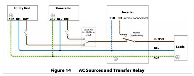
When an AC source is connected and accepted, the internal transfer relay switches to transfer the AC source power to the loads. Figure 14 shows the utility grid switch closed. The internal transfer relay has switched accordingly so that the loads receive utility power. (See the *Operator's Manual* for the inverter's acceptance criteria.)
