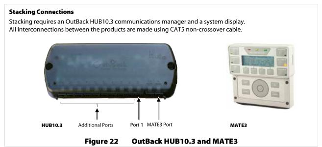
Each inverter must be assigned a stacking mode, "master" or "slave", depending on the configuration.
