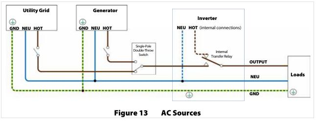
The inverter's transfer relay is normally set to provide inverter power to the output. This is shown in Figure 13, where the internal transfer relay is switched to the inverter function.
