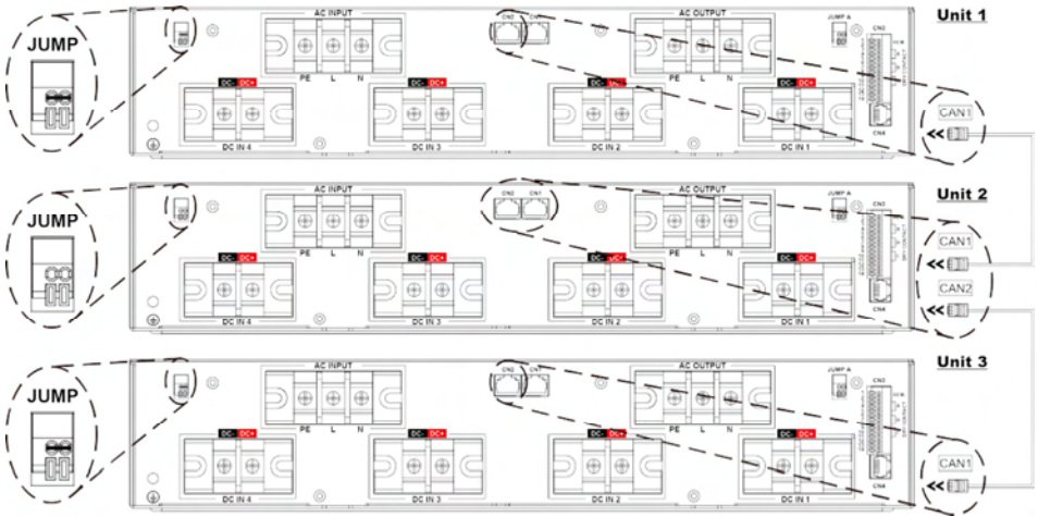
Figure 7. Parallel connection via jumper setting
