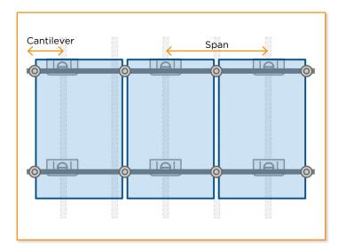
Span is measured as the distance between the centerlines of the roof attachment hardware, like a lag bolt.
