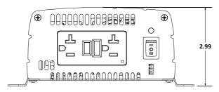
Figure 3. TS series drawing (AC output/Front View)
