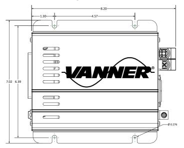
Figure 2. TS series drawing (Top View)
