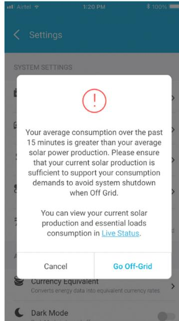
**NOTE:** If any load is set to “Basic” mode, it will remain powered off while the system is off-grid. If a load is set to “Generator” mode, it will only be powered on while off-grid if the generator is providing power to the system.
