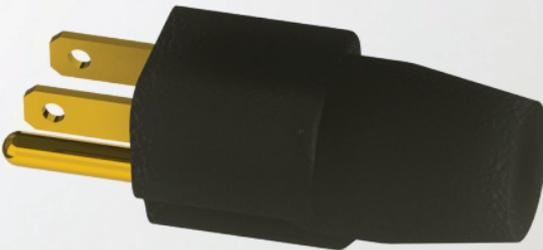
Most portable generators have a floating neutral. Surge Guard\* products will detect this as an open ground condition and not allow power to pass through. To solve this problem, insert the Surge Guard Generator Neutral-Ground Bonding Plug into a 15A receptacle on the generator control panel. This will create a neutral-to-ground bond and the open ground condition should be resolved. Please check the owner's manual of the generator to ensure the generator was designed with a floating neutral.
