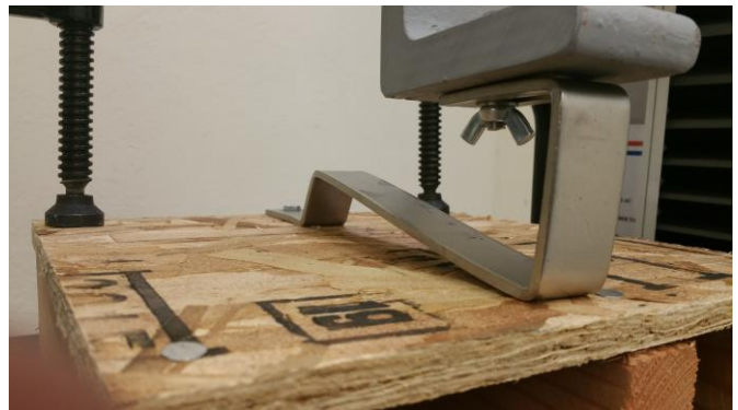
Figure 1b. Typical Failure Mode
