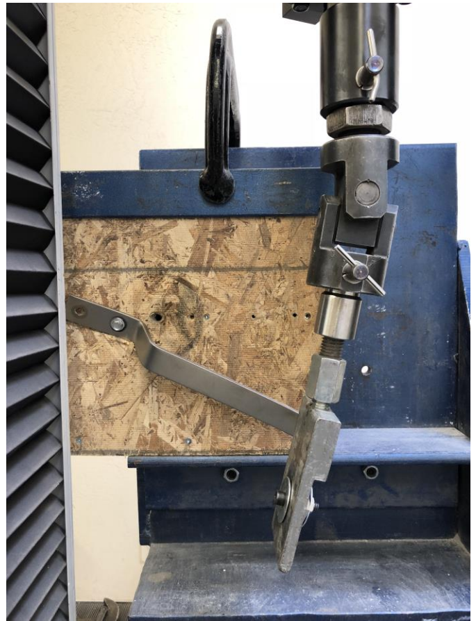
Figure 3b. Typical Failure Mode
