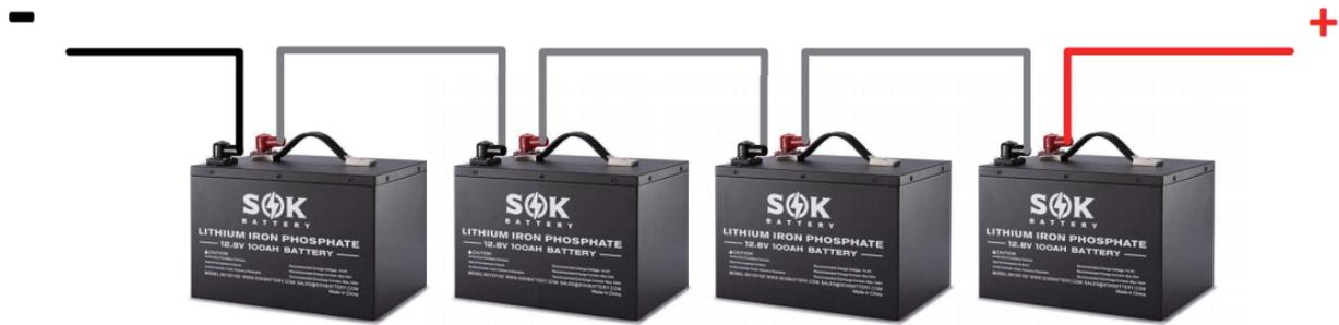
※ **Important points to note when connecting batteries in series**
