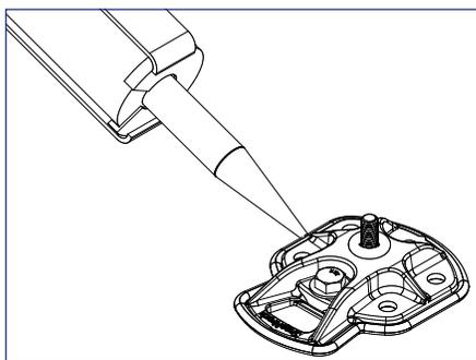
**8) Apply a 1/4" bead of ChemLink M-1 roofing sealant to base of 5/16" threaded stud & to the entire perimeter of OmniBase™. Clean all smooth substrates with isopropyl or denatured alcohol a minimum of 2" all around OmniBase™. Brush away all gravel or loose granules to the same distance.**
