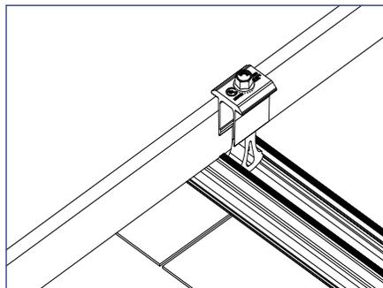
2) Slide the clamp flush to the module with the top lip of the mid clamp over the top edge of the module frame.
