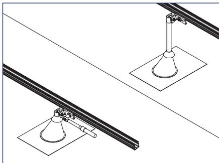
14) Set rails into the Ultra Rail Mounting Hardware on front and rear mounts then tighten the Ultra Rail Mounting Hardware to 12 ft-lbs. Connect multiple lengths of rail using the Ultra Rail Splice (see "UR-40 or UR-60 Rail Splice" sections of manual)
