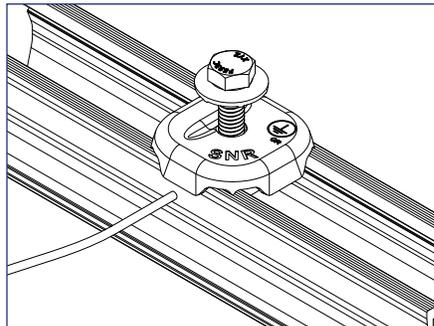
2) Place grounding conductor into slot underneath the washer.
