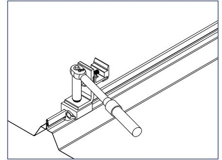
3) Torque black seam clamp bolt to 15-16 ft-lbs.
