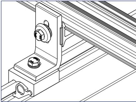
4) Ensure rotation lock is properly aligned with Ultra Mount and L foot during rail installation.
