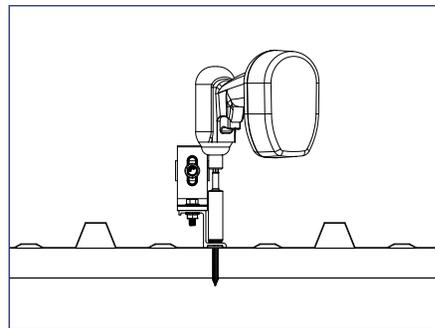
2) Determine the location of the supporting structure of the roof. When possible, secure the VersaBracket using all hole locations; when not possible, always use the two upslope hole locations. The only surface preparation necessary is to simply wipe away excess oil and debris.
