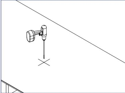
1) If required for rafter/truss applications; using roof attachment locations drawn on roof during system layout, drill pilot hole(s) into roof framing member.
