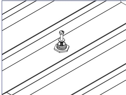
2) Attach the base with 5/16" lag screw (or 1/4" self-drilling screw for metal structures), drive screw for minimum 2.5" embedment into the roof framing member.
