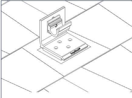
1) Using roof attachment locations drawn during system layout (refer to “Pre-Installation Requirements”), check positioning of UltraFoot™, Deck for proper alignment on shingle course.
