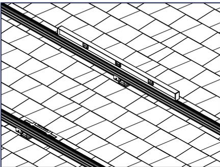
4) Level the top rail by moving the string line down the length of the rail, matching pitch over the entire length of the array.
