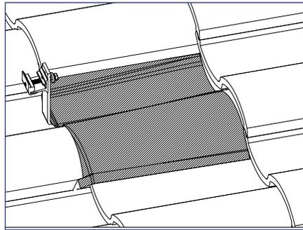
10) **OPTIONAL:** Install Tile Replacement flashing in place of roof tile over tile hook. Flat, W, and S, tile replacements are available.
