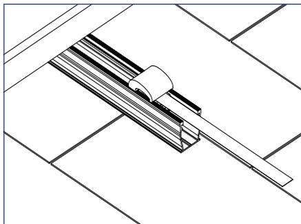
1) Slide the preassembled Universal End Clamp (UEC) into the end of the rail.
