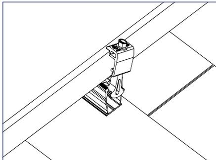
1) Snap the end clamp base into the top channel of the rail.
