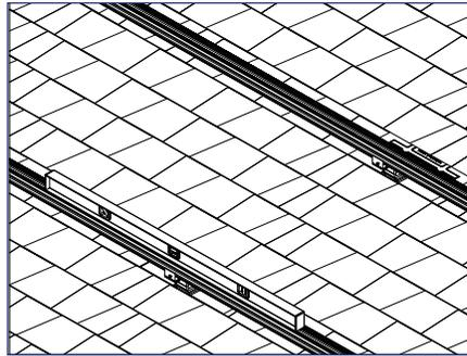
2) Level the bottom rail of the array to the roof and tighten attachment points.
