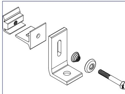
2) Re-assemble Ultra Rail Mounting Hardware components onto roof attachment in the following order:
