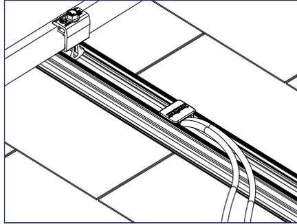
2) Install the Wire Retention Clip by snapping it into place on the rail.
