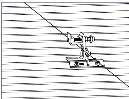
2) To ensure brackets are correctly aligned, install a single ProteaBracket on each end of the roof at a measured, consistent distance from the bottom edge of the roof. Use a string line between the two brackets. Mount the remaining ProteaBrackets along the string line. For upslope bracket-spacing techniques, reference the S-5! website at [www.S-5.com](http://www.S-5.com).
