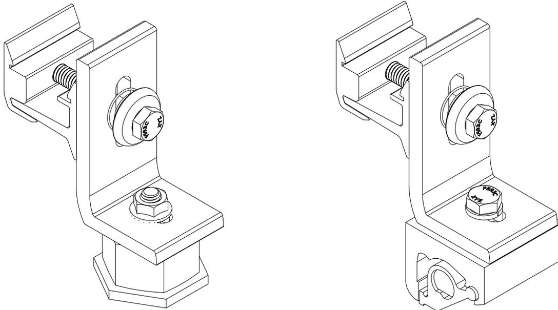
Ultra Rail Mounting Hardware Installed on Different Roof Attachments
