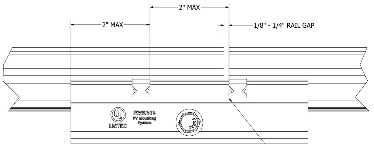
RAIL- EDGE MUST NOT PASS CLIP EDGE, AS SHOWN
