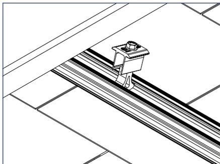
1) Snap the base into the top channel of the rail.
