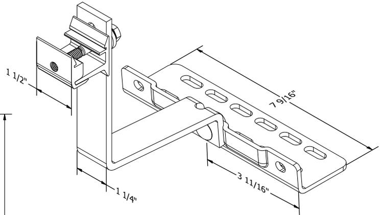
Dimensioned Ultra Rail Adjustable Tile Hook Assembly
