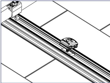
1) Snap Wire Clamp into top or side rail channel.
