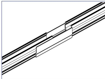
2) Slide second rail into splice, ensuring that BOTH rail flanges are engaged into lower section of splice.
