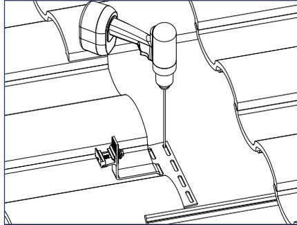
2) Align the base over the rafter so the hook can enter at the valley of a tile (W and S Tile). Drill two pilot holes through the roofing material into the roof framing member.
