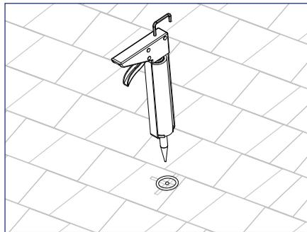
2) Apply roofing sealant in and around the pilot hole, and directly onto the lag screw to ensure a water tight seal.
