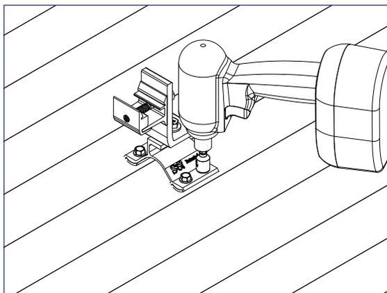
**CorruBracket must be mounted directly over & into the supporting structure of the roof, i.e. wood decking, wood or steel purlins or trusses, NEVER into the metal roofing material alone.**
