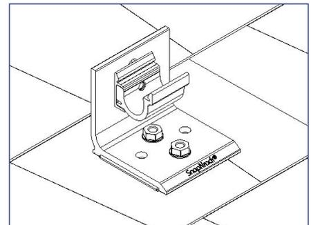
5) Optional rafter attachment step: After locating and marking rafters on the roof, use two (2) #14 wood screws to attach the UltraFoot™, Deck to rafters via the two center holes by following steps 1-3 above; no pre-drilling is required.
