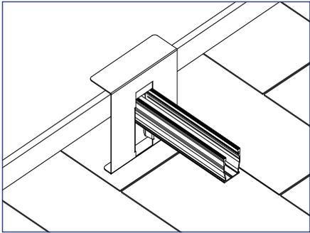
1) Slide the Rail Cutting Tool over the end of the rail and place it so that the upper lip is safely covering the edge of the module (*optional*).
