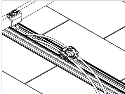
2) With Wire Clamp loose, place conductors or cables in slots.
