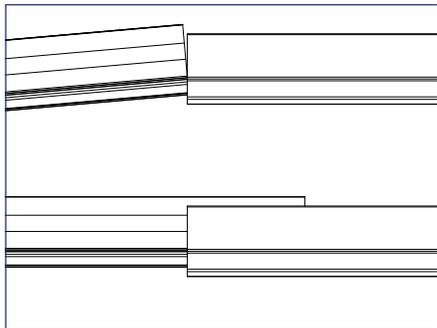
1) Slide first rail into splice, ensuring that BOTH rail flanges are engaged into lower section of splice.
