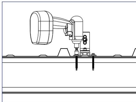
3) Install screws through the pre-punched holes in the SolarFoot into the structure below.
