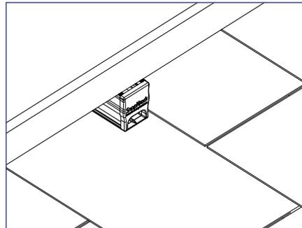
4) Insert SnapNrack Ultra Rail End Cap into the cut end of the rail to create a flush finish to the array.
