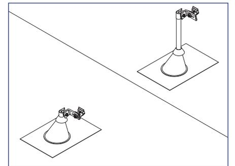
5) **Cone Type Flashings:** Install SnapNrack Ultra Rail Tilt Clamp assemblies on to Standoff Shafts.
