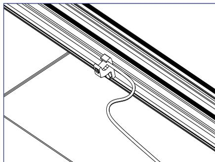
2) Place grounding conductor into slot.
