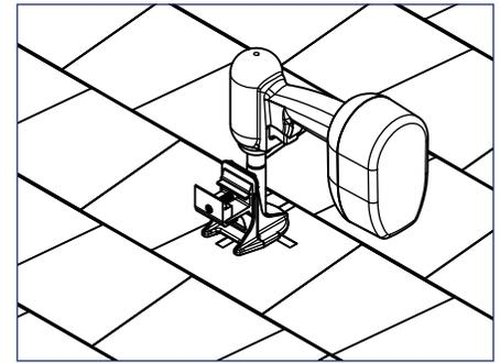
3) Insert sealing lag screw through SpeedSeal™ Foot, then drive lag screw for minimum 2.5" embedment into the roof framing member.
