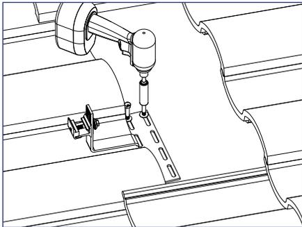
4) Attach the base with (2) 5/16" lag screws, drive lag screws for minimum 2.5" embedment into the roof framing member.
