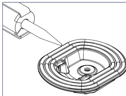
**9) Apply a 1/4" bead of ChemLink M-1 roof sealant into all 3 of the grooves on the underside of OmniShield™. Sealant should be applied as raised beads approximately 1/8" higher than the underside surface of OmniShield™.**
