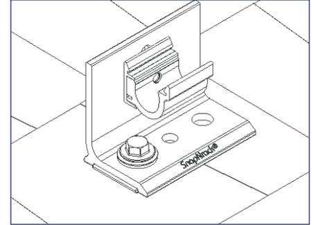
3) Insert first DeckAnchor™ screw through UltraFoot™, Anchor mounting hole and drive into roof.
