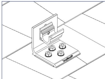
4) Repeat step 3 for remaining three wood screws. Rotate the Ultra Rail Mount to install the rail.
