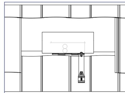
2) Peel off the backing from a 5"x13" strip of flexible flashing. Apply the strip centered laterally over the base and abutted to the Tile Hook arm. Press and roll out any creases or air bubbles with a roller to maximize contact of the flashing adhesive to 100% of the surface and base.
