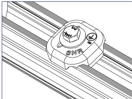
1) Snap the SnapNrack OmniLug into the rail channel on **one rail per module row**.
