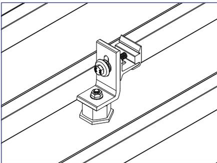
4) Attach L Foot to stud in Metal Roof Base cap and tighten hardware to 10 ft-lbs.
