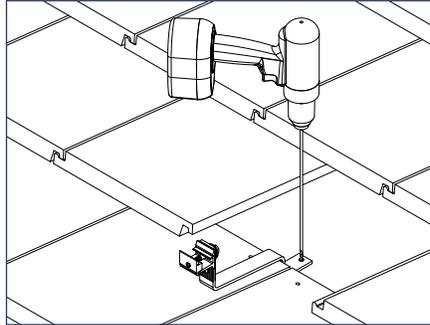
2) Align the hook over the rafter and drill two pilot holes through the roofing material into the roof framing member.
