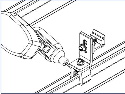
1) Position clamp and insert at desired location along the seam as shown.
