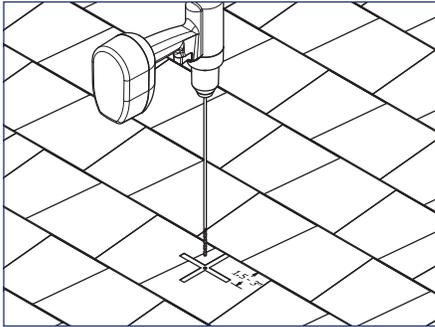
1) Using roof attachment locations drawn during system layout (refer to “Pre-Installation Requirements”), drill a pilot hole through the roofing material into the roof framing member.
