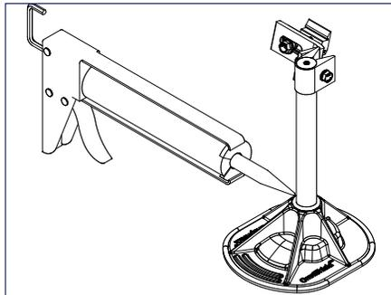
12) Apply a bead of roof sealant around the top opening of the OmniShield™ at Standoff penetration.
