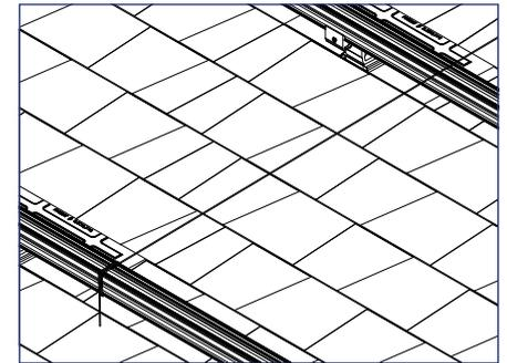
3) Run a string line or spare rail from the bottom rail to the top rail and set desired pitch of the array by adjusting the top rail, add L Foot Extension if needed.
