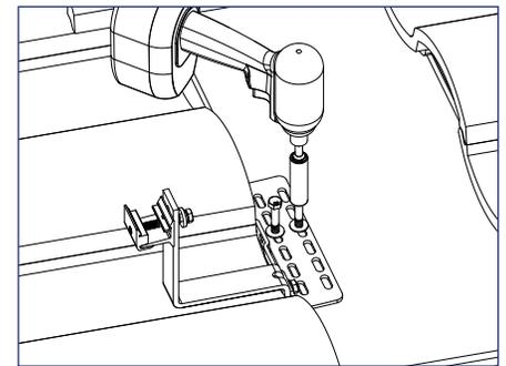
4) Apply roofing sealant to pilot holes and Tile Hook base.
