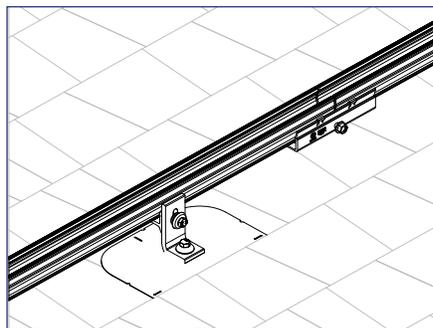
2) Install rail splice assembly onto bottom of rail, making sure both rails are seated in grooves of splice and that the splice is centered.
