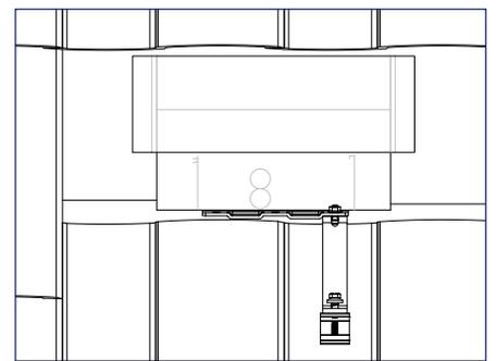
6) **OPTIONAL:** If deck mounted attachment is needed, apply roofing sealant to the hook base and position over decking in desired location.
