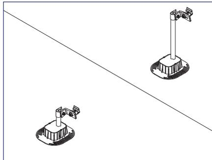
**7) Pourable Type Roof Penetration Seal System: Seal roof penetrations at bases by placing curb around Base then applying pourable sealant material.**
