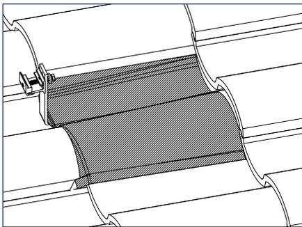
7) **OPTIONAL:** Install Tile Replacement flashing in place of roof tile over tile hook.
