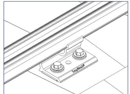
5) Install SnapNrack Ultra Rail directly to the Ultra Rail Mounting Hardware, level rails & tighten.
