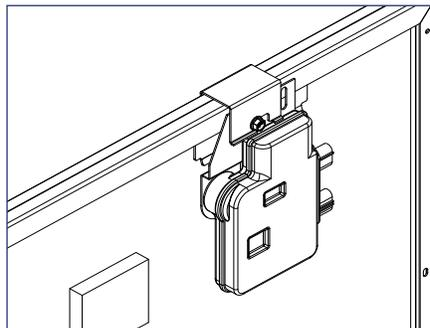
2) Slide the microinverter unit onto the bracket clamp, then move it slightly to the left.
