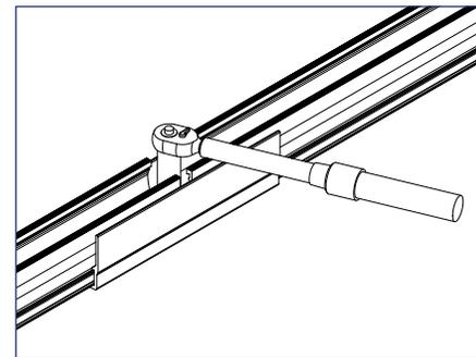
3) Tighten splice hardware to 12 ft-lbs
