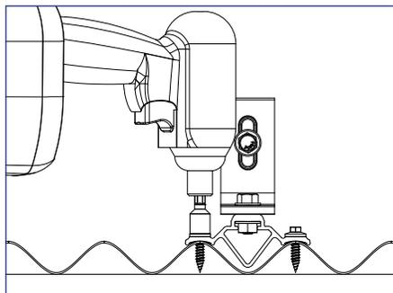
3) Determine the location of the supporting structure of the roof. When possible secure the CorruBracket 100T using all of the pre-punched hole locations; when not possible, always use the two upslope hole locations. The only surface preparation necessary is to simply wipe away excess oil and debris.
