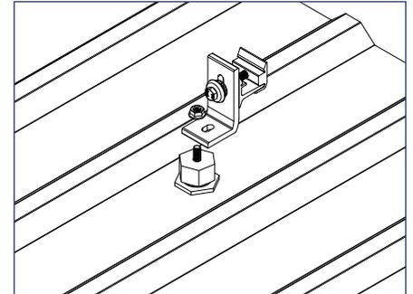
3) Thread Metal Roof Base cap onto Metal Roof Base bottom, ensuring cap is fully seated to base.
