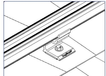
5) Install SnapRack Ultra Rail directly to the Ultra Rail Mounting Hardware, level rails & tighten.
