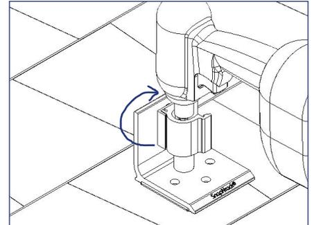
3) If needed, rotate the Ultra Rail Clamp to the vertical position for driver access. Insert #14 wood screw through the UltraFoot™, Deck and drive into roof.
