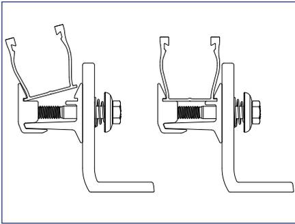
1) Set rails into the attachments by dropping and snapping into the mounts. Connect multiple lengths of rail end to end using the SnapNrack Ultra Rail Splice (see “Ultra Rail Splice” section).
