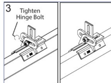
3) Before removing the protective paper over the EPDM pad, place ProteaBracket onto the panel rib and hand-tighten the hinge bolt to customize the bracket's proper fit. Because ProteaBracket is reversible, be sure all brackets on the same row have the L-foot in the same orientation and face the same way. Align carefully, peel the protective paper off the EPDM pad and adhere the bracket to the roof.
