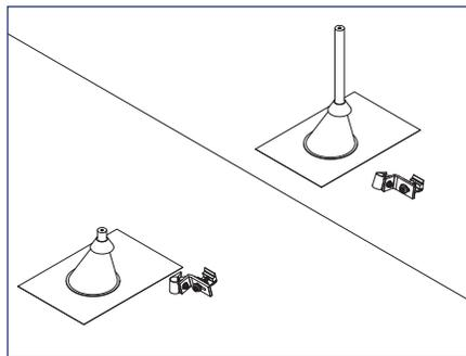
4) **Cone Type Flashings:** Install appropriate roof flashing over Standoff Shaft and seal to roof surface per roofing standards and best practices. Install Rubber Rain Collar over the Standoff Shaft.
