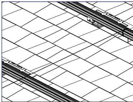
5) Level the remaining rails to the string line by working out from the middle rail, add L Foot Extensions or spacers if needed.
