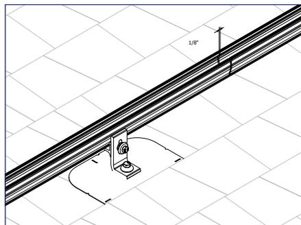
1) Align sections of rail and leave a 1/8" - 1/4" gap.
