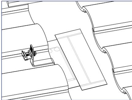
5) If deck level flashing is required, install flexible flashing per the following instructions.
