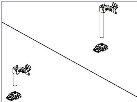
**6) Pourable Type Roof Penetration Seal System: With Ultra Rail Tilt Clamp assembly on the Standoff Shaft, install Standoff shaft onto base.**
