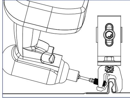
2) The clamp should be over the seam and insert as shown. Make sure the toe of the clamp engages beneath the fold of the seam as shown.
