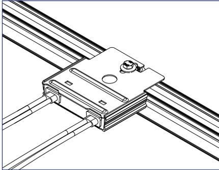
2) Install the microinverter mounting plate onto the SEMS bolt of the OmniLug.
