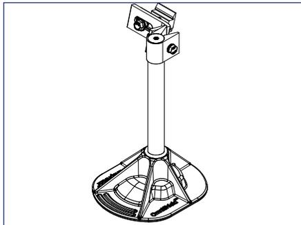
11) Install Tilt Standoff through the opening in the OmniShield™ and thread on to the 5/16" stud on the OmniBase™.
