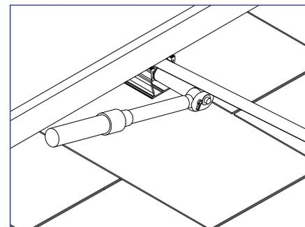
3) Use the pull tab to hold the UEC taut towards the end of the rail and tighten hardware to 10 ft-lbs.
