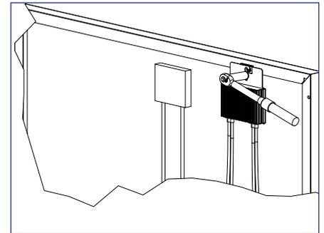
3) Tighten the mounting bolt on the MLPE Frame Attachment Kit to 10 ft-lbs.
