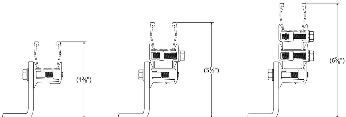
Leveling Spacer Provides Up To 2.25" of Additional Height Adjustment
