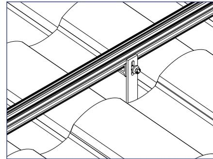
11) Install SnapNrack Ultra Rail directly to the Ultra Rail Mounting Hardware, level rails and tighten to 12 ft lbs. framing member.
