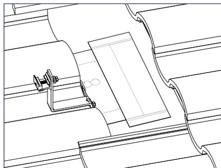
3) Peel off the backing and apply the second 4"x17" strip of flexible flashing along the top edge of the first strip with a 2" lap on either edge, then roll out any creases between the strip and the deck level surface.
