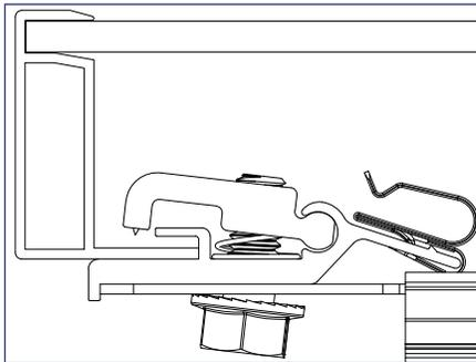
2) Position the MLPE Frame Attachment Kit on the module frame flange in a location that will not interfere with mounting system components. The module frame flange should rest against the module flange backstop on the MLPE Frame Attachment Kit.
