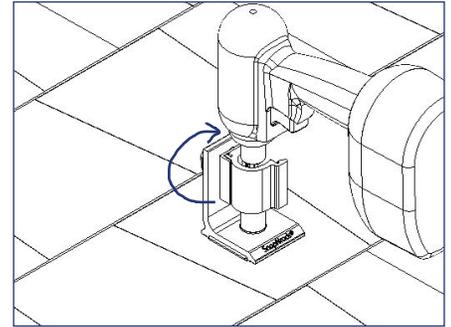
3) If needed, rotate the Ultra Rail Clamp to the vertical position for driver access. Insert sealing lag screw through UltraFoot™, Rafter then drive lag for minimum 2.5” embedment into roof framing member.
