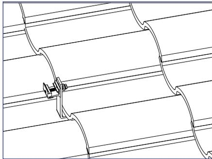
9) Using roof attachment locations drawn during system layout, remove roof tile where the roof attachment will be installed.
