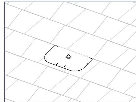
3) Pry up shingles with a breaker bar and install flashing underneath shingle course above pilot hole, and position flashing so cone is in line with pilot hole.
