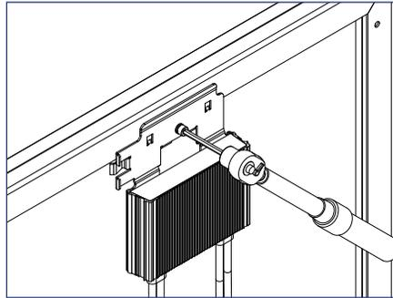
2) Install the optimizer mounting plate onto the module frame and tighten hardware to 7 ft-lbs.
