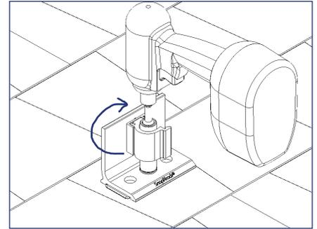
3) If needed, rotate the Ultra Rail Clamp to the vertical position for driver access. Insert sealing lag screw through the middle hole on UltraFoot™, Anchor then drive lag for minimum 2.5” embedment into roof framing member.
