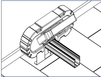
2) Use the reciprocating saw or band saw to cut off the end of the rail, then remove any sharp edges.
