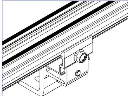
Use a single leveling spacer on no more than 30% of attachment points, and no more than two leveling spacers on more than 10%.
