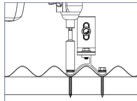
3) Secure the CorruBracket by drilling appropriate screws into the pre-punched holes and directly into the supporting structure of the roof.
