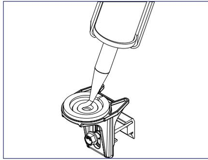
2) Fill cavity on bottom of SpeedSeal™ Foot created by sealant ring with roof sealant, as well as the pilot hole to ensure a water tight seal.
