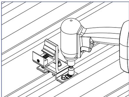
2) Peel the release paper from the base, align, and apply to roof surface so that fasteners will engage the structure below.
