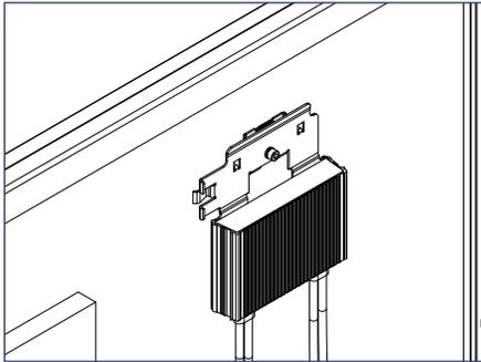
1) Locate the SolarEdge optimizer with Frame-Mounted Module Add-On at a location on the module frame that will not interfere with the SnapNrack rail.
