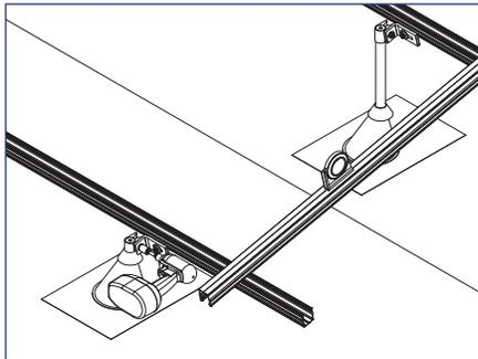
15) Set all Ultra Rail Mount angles to desired tilt angle using an Inclinometer tool or other pitch measuring device. Tighten bolts to 10+ ft-lbs.
