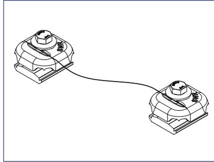
*Example of assembled bonding jumper using (2) SnapNrack OmniLugs*
