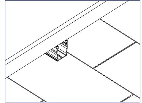
3) Remove the Cutting Tool from the rail, then remove any sharp edges.
