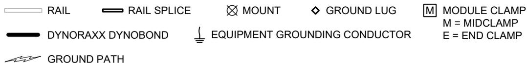
R/C (QIMS2), DynoRaxx (E357716) photovoltaic bonding jumper cat. no. DynoBond is an optional component that may be used with this system. The DynoBond jumper has been evaluated to provide module to module bonding. The DynoBond device attaches to the frame flange of adjacent modules.
