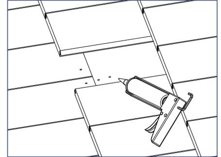
3) Apply roofing sealant to pilot holes and Tile Hook.
