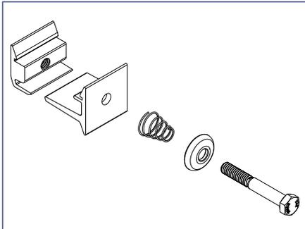
1) Disassemble Ultra Rail Mounting Hardware components, taking note of their installation order and orientation.
