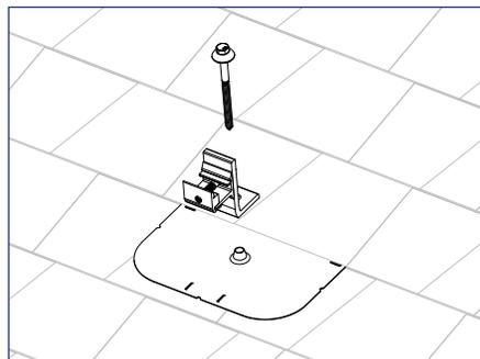
4) Insert Umbrella Lag Screw through Umbrella L Foot and cone in flashing, then drive lag screw for minimum 2.5" embedment into the roof framing member.
