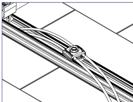
4) 4-Wire Clamp intended for PV Wire conductors, Trunk Cable Clamp intended for trunk cables, Universal Wire Clamp intended for both PV Wire conductors and AC trunk cables.
