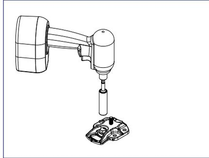
2) Apply roofing sealant to underside of OmniBase™ & in pilot hole(s). Attach Base to roof with the appropriate fastener/s based on application from the list below:
