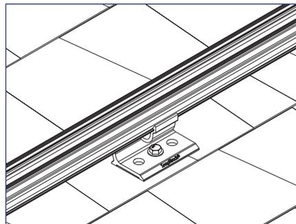
4) Install SnapNrack Ultra Rail directly to the Ultra Rail Mounting Hardware, level rails & tighten.
