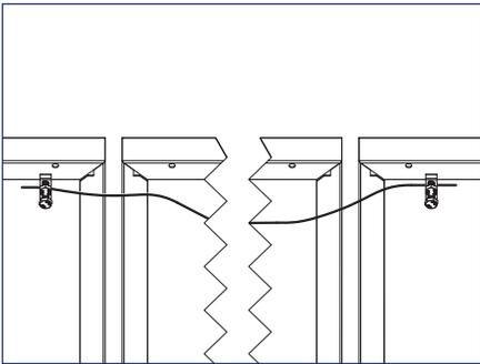
3) Before the module is removed, attach the assembled bonding jumper. Depending on where the module will be removed and choice of ground lug, jumper attachment locations will vary.
