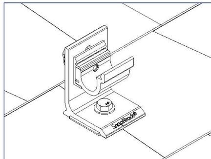
4) Rotate the Ultra Rail Clamp to install rail
