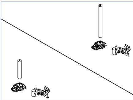
3) **Cone Type Flashings:** Install Standoff shaft onto base.
