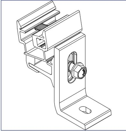
1) Snap leveling spacer into Ultra Rail mount.
