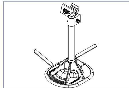
13) Smooth out the excess roof sealant at the base of the OmniShield™ and at the top opening.
