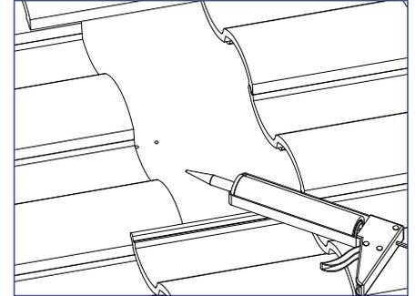
3) Apply roofing sealant to pilot holes and Tile Hook base.
