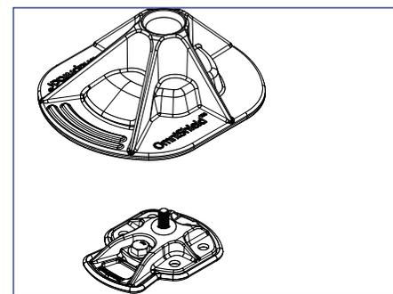
**10) Install OmniShield™ on to roof over the OmniBase™, pressing firmly onto roof until sealant can be seen around the base of the OmniShield™.**
