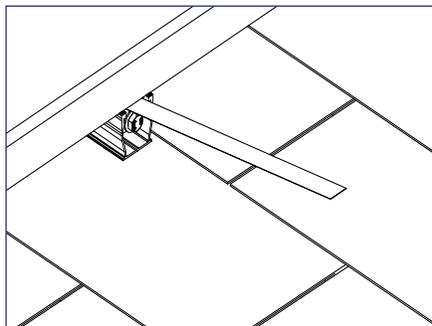
2) Lift the module and slide the clamp far enough under the module to pass the lip of the bottom edge of the module frame.
