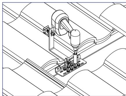
5) Attach the base with (2) 5/16" lag screws, drive lag screws for minimum 2.5" embedment into the roof framing member.
