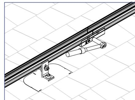
3) Tighten splice hardware to 12 ft-lbs.
