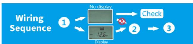
Connect the system in this order **①** Battery first. Once the battery is connected, the LCD will turn on. If LCD is not on, stop connecting, and check whether the positive and negative poles are connected correctly. Only after the LCD is on can you continue to the next step. Always connect the battery first, this allows the controller to recognize the system voltage **②** PV array **③** Load. Disconnect the system in the reverse order **③ ② ①**.
