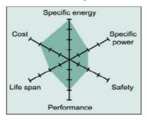
Lithium Nickel-Manganese Cobalt Oxide (NMC) LiNiMnCoO<sub>2</sub>
