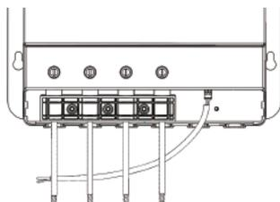
Secure the Temperature Sensor lug to one of the battery posts
