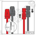
Bind the Anderson PP75 connectors by sliding the side grooves.
