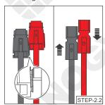
Bind the Anderson PP75 connectors by sliding the side grooves.
