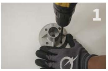
Locate the desired mount placement using the QBase as a template, mark the required penetration points with either a pen or light drilling.
