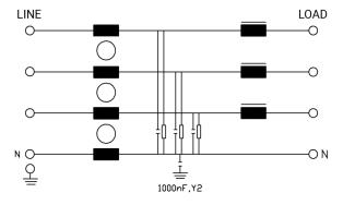
Connect both Enphase IQ Gateway and Enphase microinverters on the array or load side of the filter and wire the utility feed to the line side of the filter.
