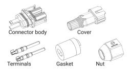
MARNING: Risk of equipment failure. Do not mix male and female connector parts when assembling connectors.
