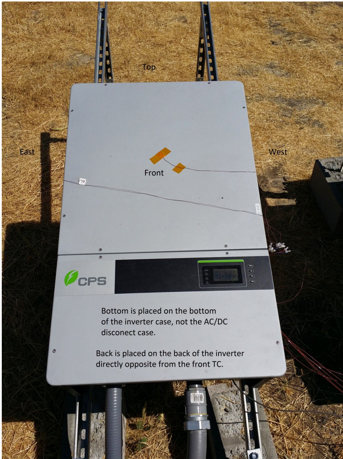
Figure 2 Image indicating thermocouple placements
