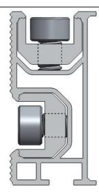
4. The corrugated surfaces on both rails and roof hooks ensure the secure connection of these parts. The loop design maximizes and distributes rail strength evenly throughout the length of the rails. The rails have three openings, which make them compatible with a large variety of roof hooks.
