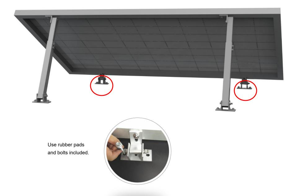
4. Adjust the length and tilt of rear legs to desired angle, tighten side bolts and mount to flat surface.
