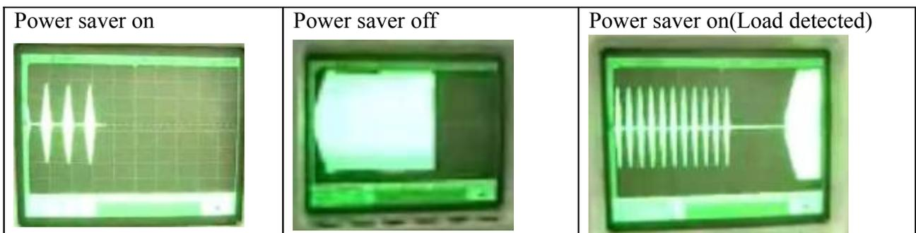
Note: The minimum power of a load to take inverter out of sleep mode (Power Saver On) is 25 Watts.
