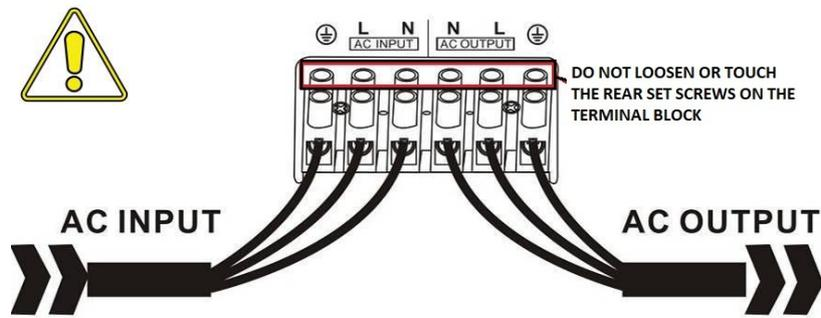
**Do not loosen or touch the rear set screws on the terminal block.**
