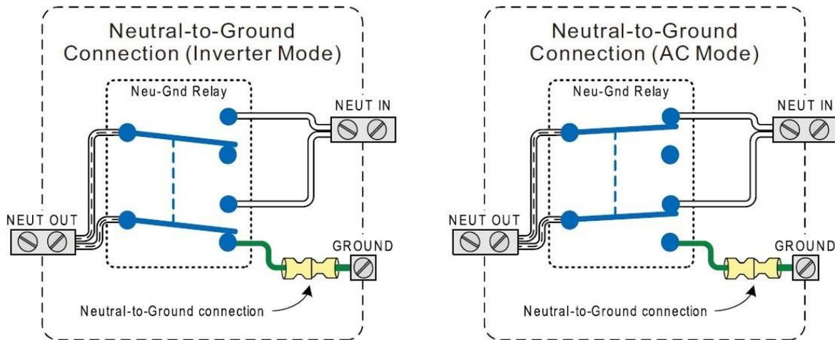
This design avoids two neutral-to-ground connections from existing at the same time, thereby preventing an electrical shock hazard between the vehicle/boat's neutral and the external AC source's neutral.
