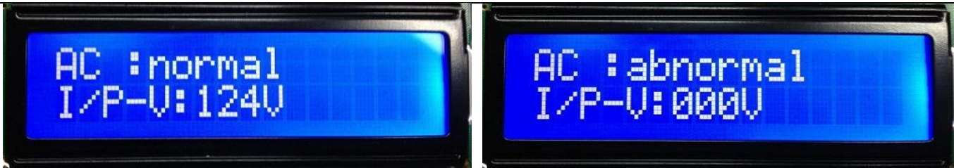
AC Status & Input Voltage
