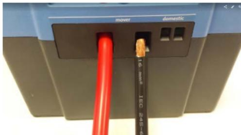
Because of the high currents involved when operating the mover, a careful installation of the cables is crucial. Improper connections of the cables can cause loss of performance, overheating and damage. The Victron PPP is equipped with high-power terminals that can provide a reliable connection on fine stranded wire ends. High quality eyelets and specialist crimping tools are therefore not needed. Solid wire or wires with thick strands will not provide a proper connection.
