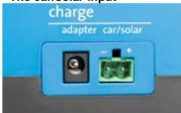
A 11 to 20 VDC power source can be connected to the car/solar input, to charge the PPP from the towing car electrical circuit, a 12 V solar panel or a 12 V battery. When connecting to a car trailer plug, the used contact must be carefully selected, not to overload any circuit or to over discharge the car battery.
