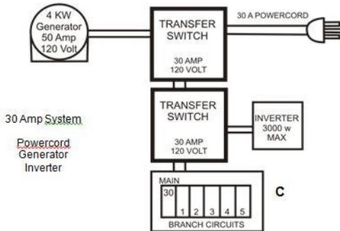
Diagram 2 – Typical Generator inverter / Alternate Source Connection
