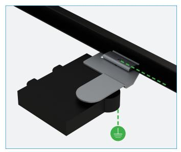
The MLPE Mount's bolt and bonding pin establish bonding between MLPE Mount and module. It is Single Use only.
