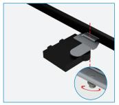
ENGAGE MLPE & MOUNT ONTO MODULE FRAME FLANGE AND TIGHTEN Required Torque - 20ft-lbs
