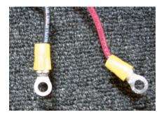
Ring lugs are included to allow easy installation of the MNSPD. If they are to be used, then you would need to strip the wire, push it into the barrel of the ring lug and crimp the barrel with an appropriate crimper. Make sure to pull on the wire after crimping to verify that the crimp is adequate.
