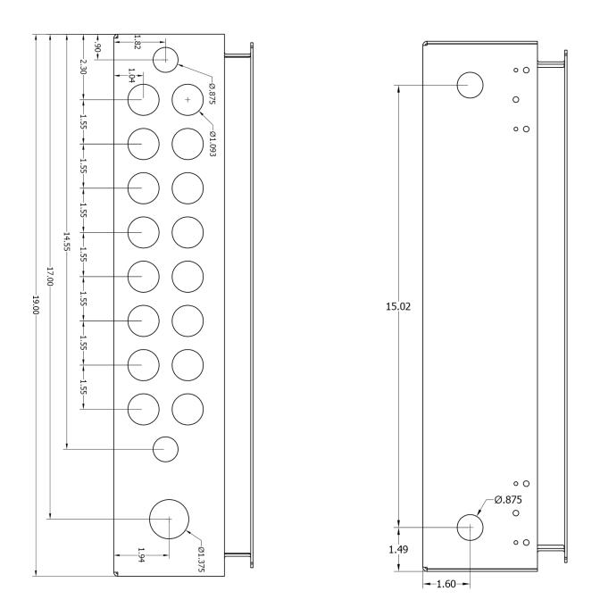
MNPV16HV Bottom and side knockout location and size No Scale
