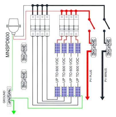
Here the Combiner is set up as two separate four string combiners. One section combining the Positive side of the strings and the other combining the negative side. Both sides are disconnected at the same time.
