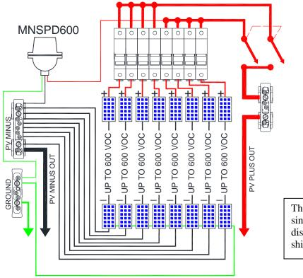
The parallel setup gives you a single 8 position combiner with disconnect. This is the default as shipped configuration
