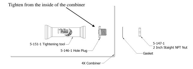
Hole plug parts placement on Type 4X Chassis
