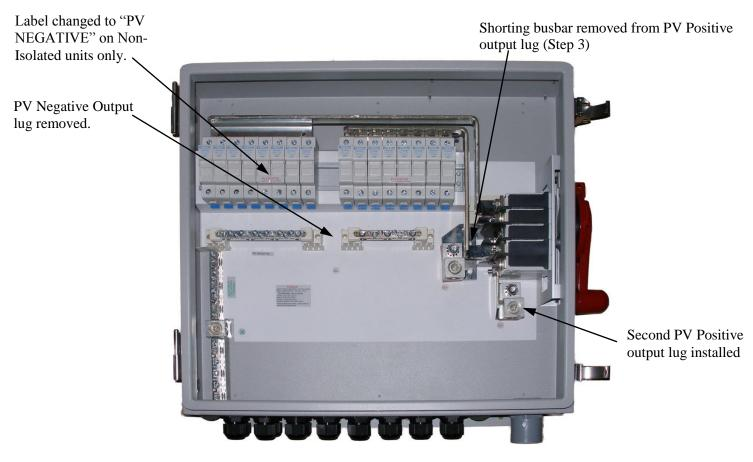
MNPV16HV Configured for 2 Inverters / Non-Isolated
