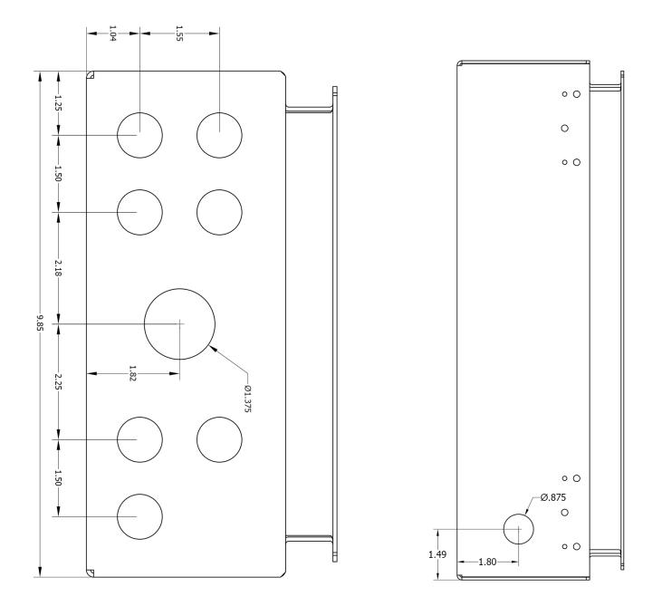
MNPV6HV Bottom and side knockout location and size No Scale
