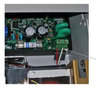
**Step 7**: Strip one end on the red and white wires included in the kit <sup>1</sup>/<sub>4</sub>" and connect them as shown with the red wire on the left side of the terminal block marked "PV+" and the white wire on the right side marked "PV-". Route the wires downward under the large switch.
