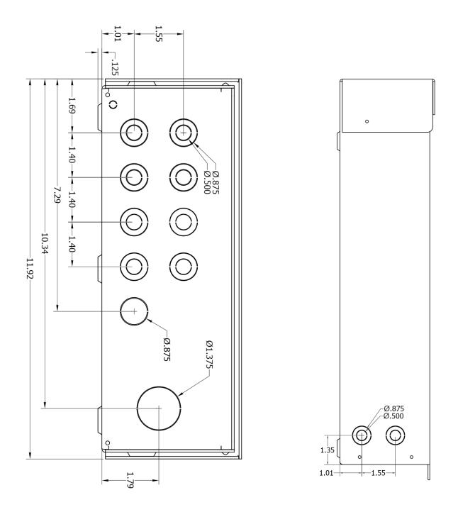
MNPV8HV Type 3R Bottom and side knockout location and size No Scale
