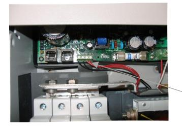
**Step 6**: Connect the two black wires to The left side of the terminal block marked "BK1" and "BK2". Connect the two red wires to the right side of the terminal block marked "S1" and "S2".
