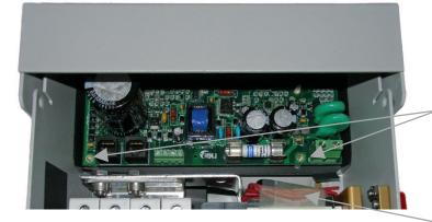
**Step 5B**: Secure board with 6-32 screws (2).
