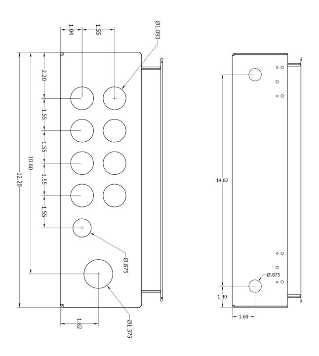
MNPV8HV Type 4X Bottom and side knockout location and size No Scale
