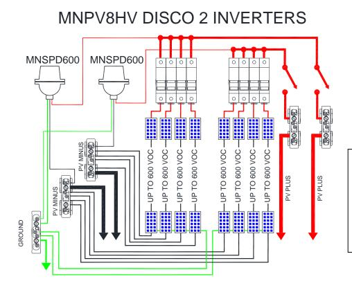
This arrangement allows the 8 position combiner to act as two separate 4 position combiners that disconnect together. Note that the second MNSPD600 is sold separately.
