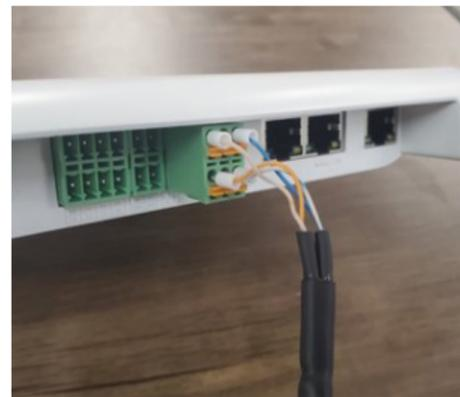
3. One of your eFlex batteries will have a plug in the port marked "CAN RS485".
