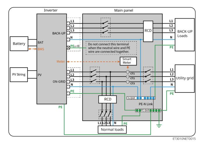
N and PE cables are separately wired in the Main Panel.
