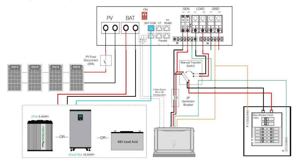
WARNING: Make sure to turn off the Generator Breaker on the Envy before turning on the Generator and the PV system is bypassed. Fault or Damage will occur if power enters to the load side of the Envy.
