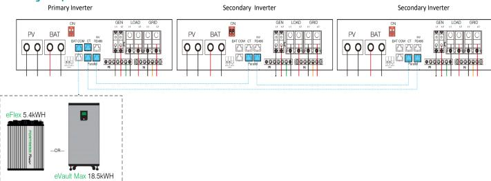
Use the Communication Cables included in the in the Envy Inverter along with those of the eFlex5.4kWh and eVault Max 18.5kWh.
