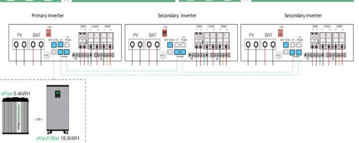
When paralleling multiple Inverters, make sure to complete paralleling process by identifying which is the Primary inverter and the secondary on Parallel System area under the Advance Section. You can confirm by Selecting the Home Icon and view how many inverters are in connection **(PNUM)** and which **Role** each has **(P=Primary, S=Subordinate)**
