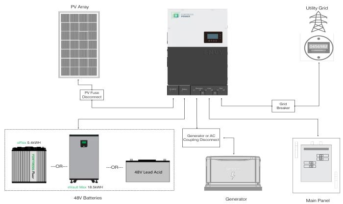
Please include the following recommended breakers for each system connection in accordance with the local jurisdiction. Battery breaker and Load breaker are already integrated in the Envy inverter.
