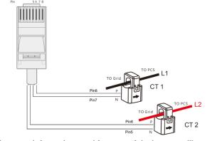
pointing to the inverter. (\*\*\* Incorrect install of the CT will cause The Display to show incorrect information's and features of the inverter will not function correctly) If the CT are in a wrong direction, there is an option you can change the direction of the CT on your inverter call: CT Direction Reversed (Only for Direction not CT1 or CT2 Placement) in Advanced Tab of the LCD. You would not need to go change it physically.
