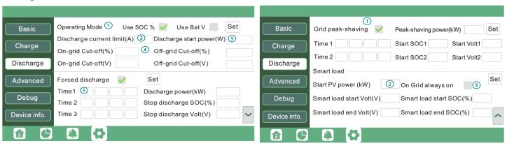
Figure#NameFunction1Operating ModeYou can choose "Use SOC %" or Use Bat V" to control the battery discharge state
