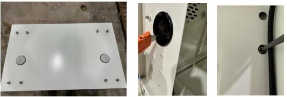
Set the upper inverter cabinet on top of the lower cabinet and then affix the two cabinets together using provided 8 attachment screws. **Do not perform this step with the batteries or inverters inside the cabinet.**
