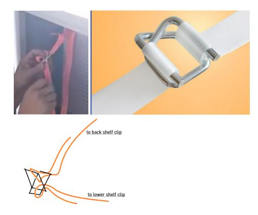
iv) Lace the stability buckle through the orange strap and tighten.
