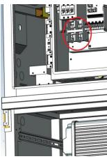
conductor runs 10' or less, or up to 4/0 maximum. Note: if using 4/0 cable, check terminal lug width to ensure compatibility with inverter port. UL battery cable is recommended. DLO cable can be used, but is difficult to bend in the space provided. If using parallel conductor runs to an inverter (Ex. Envy 12k, Sol-Ark 15k configurations), use 1/0 cable minimum when running parallel power conductors to the inverter. Do not use larger than 2/0 cable for parallel runs.
