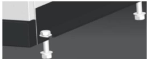
A 3" concrete pad or greater is recommended but strength of pad is dependent on sub-base / location. The M10 expansion bolts have a 12mm sheathing so a ½" masonry drill is necessary. Drill approximately ½" deeper than the intended depth of the sleeve anchor bolt, at least 1.5" deep, and use a hammer drill to drive the anchors into place, positioning the nut on the bolt as to protect the threads when driving into place.
