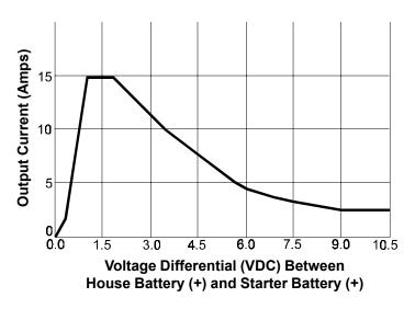
The graph shows the relationship between the voltage difference over the echo-charge (voltage difference between house (+) and starter (+) battery) and the charge current.
