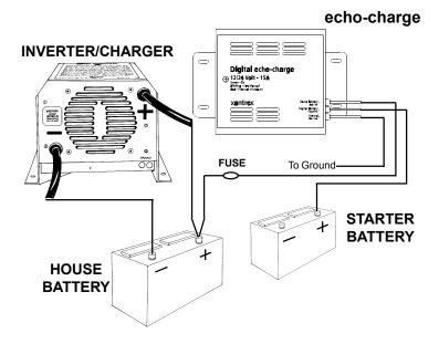
When the input voltage is 13.0/25.5 volts DC or higher, echo-charge automatically switches ON. The LED glows a steady green. When the input voltage is lower than 13.0/25.5 volts, the echo-charge automatically switches OFF, and the LED blinks green. The output voltage of echo-charge is limited to 14.4/28.8 volts. When it reaches 14.4/28.8 volts, the charge current will decrease, maintaining a float condition. The starter battery will be fully charged without overcharging.
