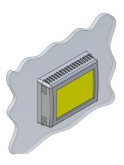
**Step 5:** Aligning the buttons with the holes in the back of the display. Press the display against the wall and gently slide the display down to lock it in place.
