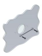
**Step 1:** Locate the mounting buttons horizontally across the hole with the smaller diameter against the wall.
