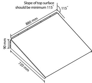
Fig. 3.1(a) Dimensions of Drip Shield
