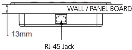
The thickness of the wall/panel board at the place of mounting should not be more than 13mm to ensure that the RJ-45 jack opening is not obstructed.
