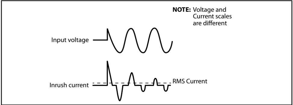
**Fig 1.2** Inrush current in an SMPS
