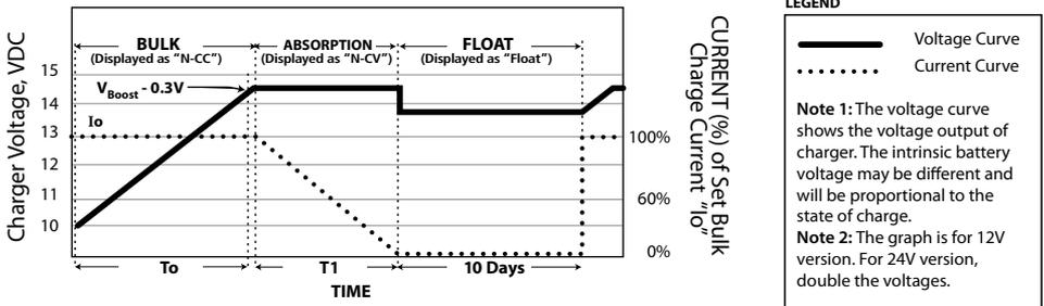
Fig 5.1 Charging Curve for Normal 3 Stage Charging
