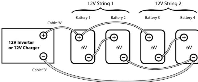
**Fig. 3.7 Series-Parallel Connection**
