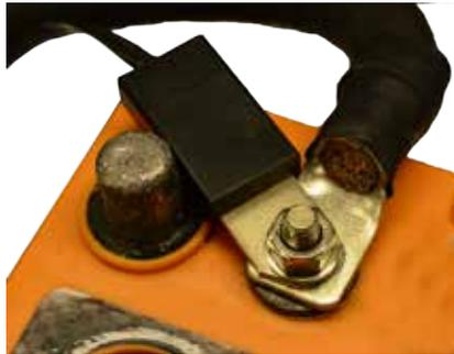
Fig 2.5(b) Temperature Sensor Installation
