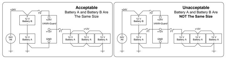
In certain applications, such as private coach or alternate energy applications, it may be desirable to have additional 12 volt "House Batteries" to operate heavy 12 volt (inverter) loads. Use the VANN-Guard to charge the additional batteries.
