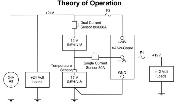
In many 24 volt electrical systems it is desirable to tap into the battery system to obtain power for 12 volt loads. This method, while seemingly simple, causes a charge imbalance resulting in Battery B (see diagram) being overcharged, and possibly boiling, while Battery A discharges.
